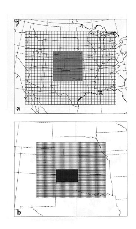
Figure 4.2 a) Nested grid setup for Case 980726 in RAMS with grids 1 and 2; b) nested grid setup in RAMS with grids 2 and 3.
