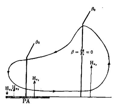
Figure 2.1 A typical PIMS vertical cross section over land. PA represents an area with reduced surface sensible heat flux (positive  $H_{s1}$ ,  $H_{s2}$ ) compared to surrounding ( $H_{ss}$ ). In some cases, the surface sensible heat flux of PA might even be negative ( $H_{s3}$ ). Over PA, a suppressed convective boundary layer or occasionally even a stable boundary layer, occurs over PA as compared to surroundings. Taken from Segal and Arritt (1992).
