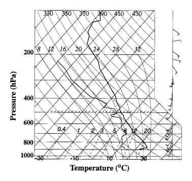
Figure 4.4 Skew T-log p diagram for temperature (°C), dew point temperature (°C), and wind (m s<sup>-1</sup>) on 1200 UTC 26 July 1998 at Amarillo, Texas ('X' in Fig. 4.3). A full (half) barb is 5 (2.5) m s<sup>-1</sup>. Data was obtained at NCAR mass storage.
