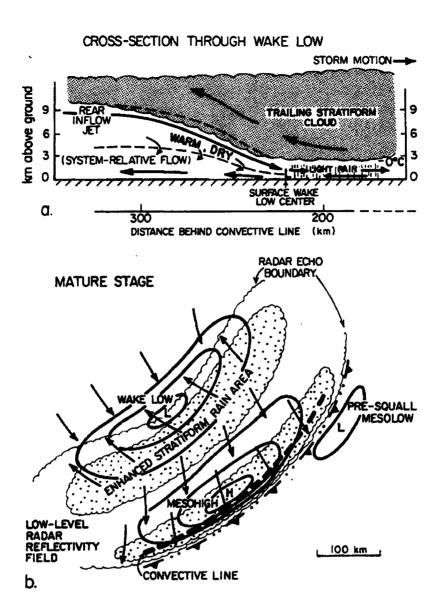
Figure 2.2 a) Schematic cross-section through wake low; b) surface pressure and wind and precipitation of a mature squall line; Dashed line in (a) denotes zero relative wind. Arrows indicate streamlines, not trajectories. Taken from Johnson and Hamilton (1988).
