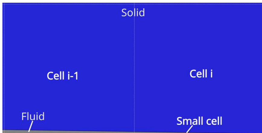
Figure 3.3: Two cut cells with the right having a small fluid portion, illustrating the small cell problem.
