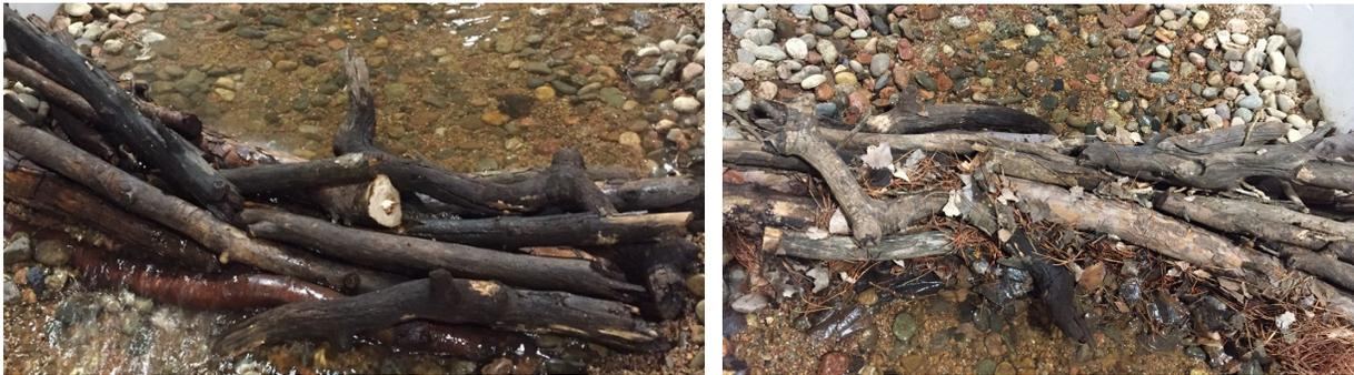
**Figure 2.8.** Comparison of visual porosity with LW only (high porosity, at left) versus LW, twigs, and CPOM (low porosity, at right).
