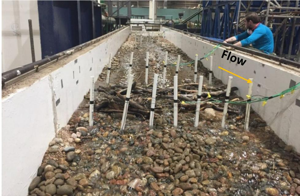
**Figure 2.4.** Flume configuration set for IRIS. Electrodes attached to PVC are connected by wires to the IRIS to image the subsurface flow.
