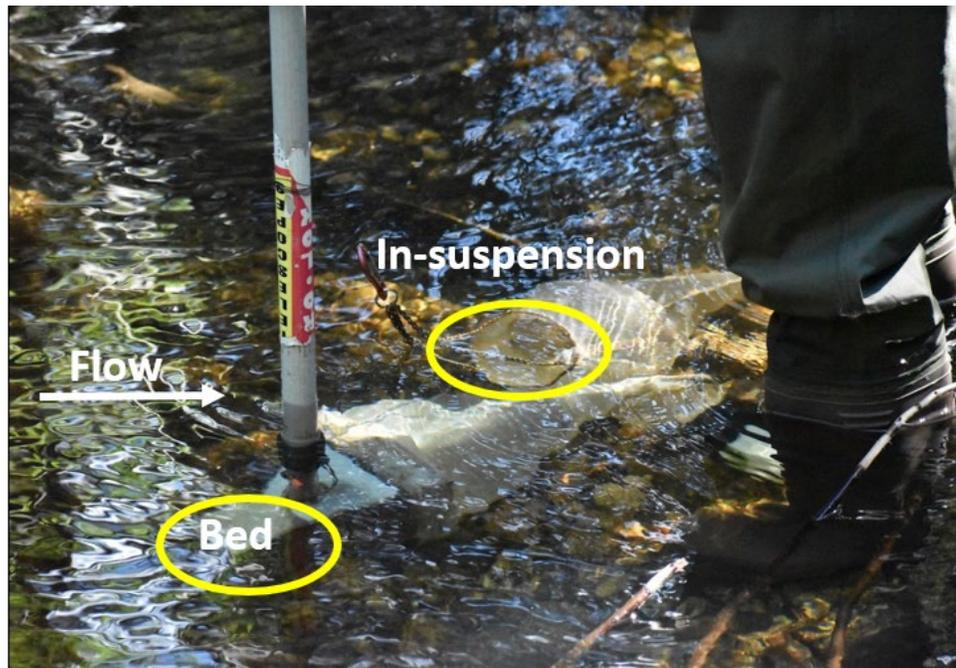
**Figure 3.2.** Helley-Smith bedload sampler and surface seine with expanded orifice used for CPOM sampling at surface, midpoint, and bed depths. Three nets were used at high flows at surface, midpoint, and bed depths and only surface and bed nets were used at low flows. This photo, taken at base flow, shows surface and bed nets.
