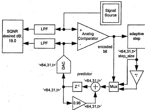
Fig. 3. Adaptive delta modulator for speech coding.
