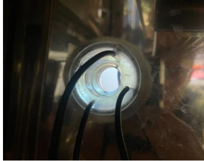
Figure 26. The custom incubator plug is installed into the access hole from the inside of the incubator. The four cords are sealed around the perimeter of the filter hole (filter not shown).
