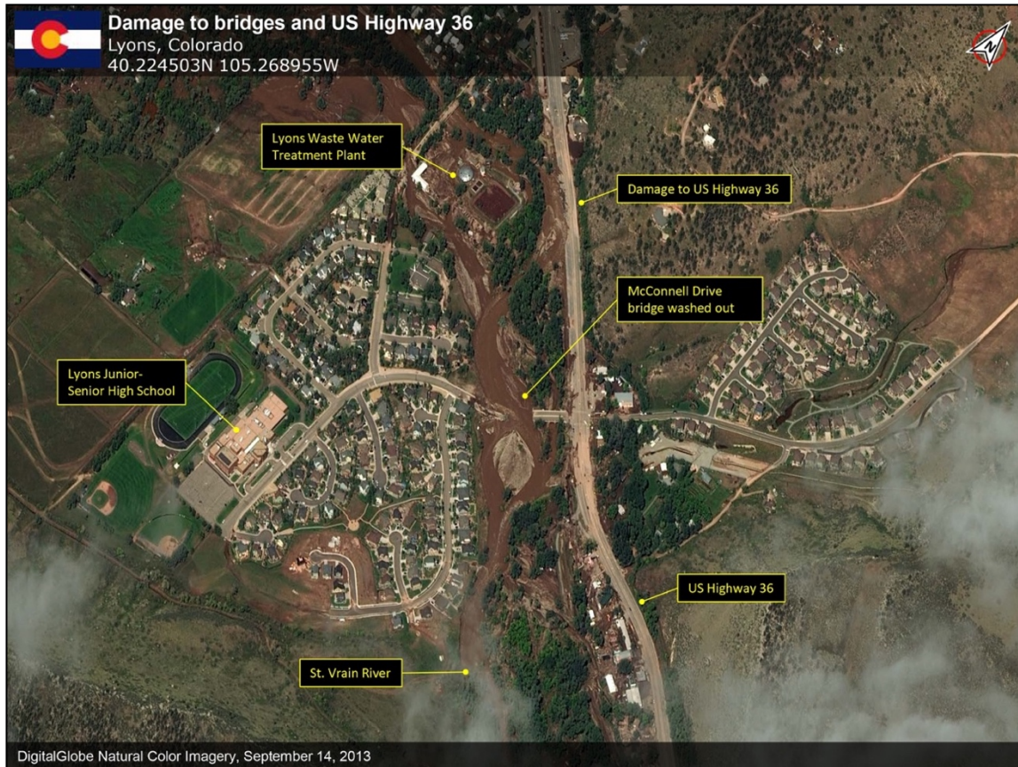
Figure 1.4 Aerial Photograph of Bridge and Road Damage Due to Rivers Re-routing During the 2013 Floods
