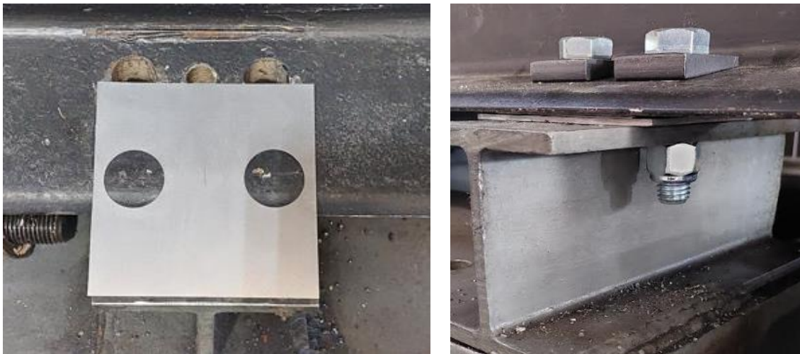
Figure 60. Example of engine shim cut from shim stock, and one completed mounting point.
