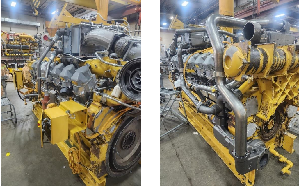
Figure 49. G3516J engine after rebuilding and before new paint.
