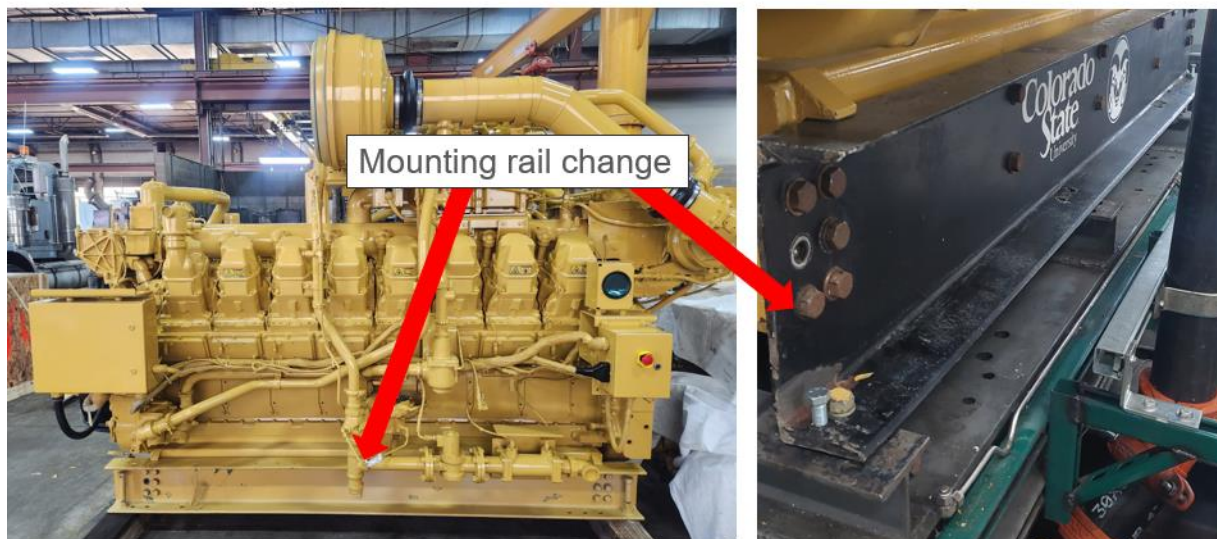
Figure 58. Before and after the mounting rails on the G3516J engine were replaced.
