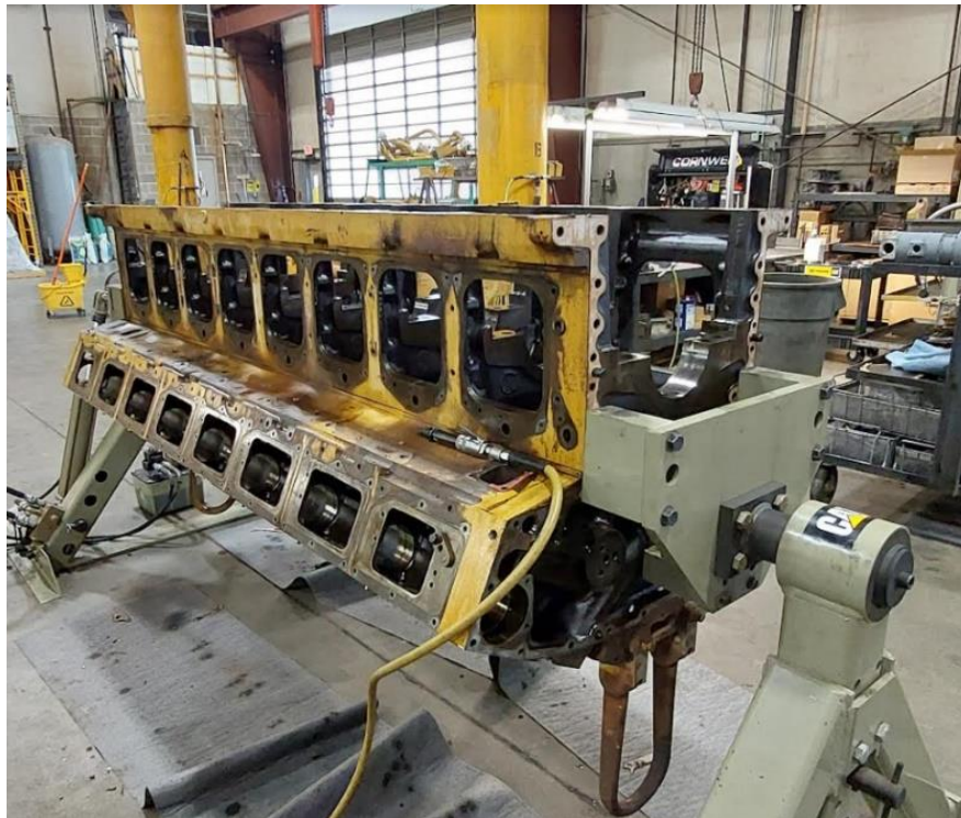
Figure 48. G3516J engine block after disassembly.
