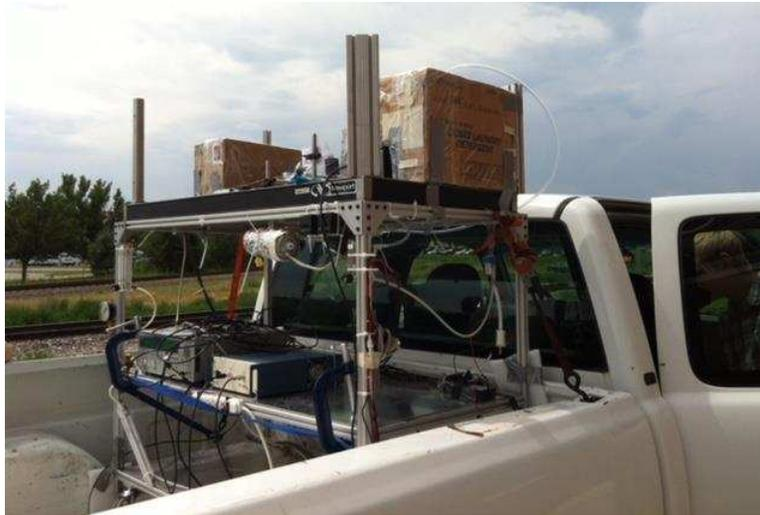
Figure 4.7: Sensor Phase-I mounted in bed of pickup truck for preliminary mobile tests.
