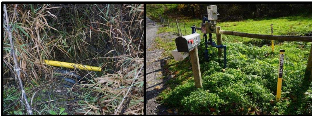
Figure 6.27: (Left): Pipe where potential leak was measured ( $< 3$  ppmv) on 10/29/17. (Right): Valve box or pipes where potential leak ( $< 12$  ppmv) was measured on 10/31/17.
