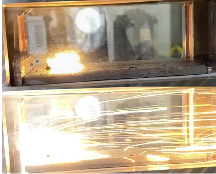
Figure 3.7: Laser Stabilized Flame (Top) and Flair up Event (Bottom)
