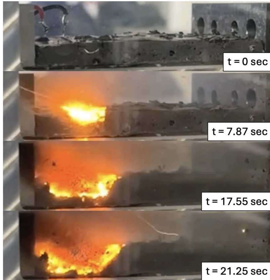
Figure 3.11: Regression of fuel grain using grain group five inside of a three inch cavity
