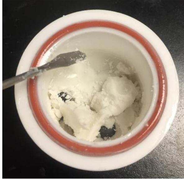
Figure 22. Dried HAp resin in milling jar with black agate milling balls.
