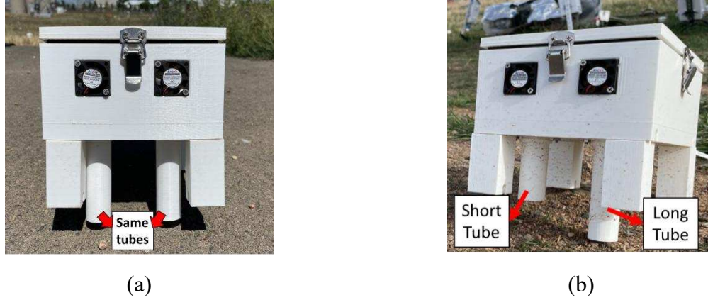
Fig. B. 3. Side views of the natural gas detector on (a) the asphalt area and (b) the soil and grass area. The detector on the asphalt area has two short open tubes of the same lengths. Both tubes connect to natural gas sensor (TGS) to measure surface methane concentrations. (b) The detector on the soil and grass area with one long and one short open tube. The short tube is responsible for measuring the surface methane concentration, while the long tube is responsible for monitoring the near-surface methane concentration at the depth of 1.2 cm below the ground surface.
