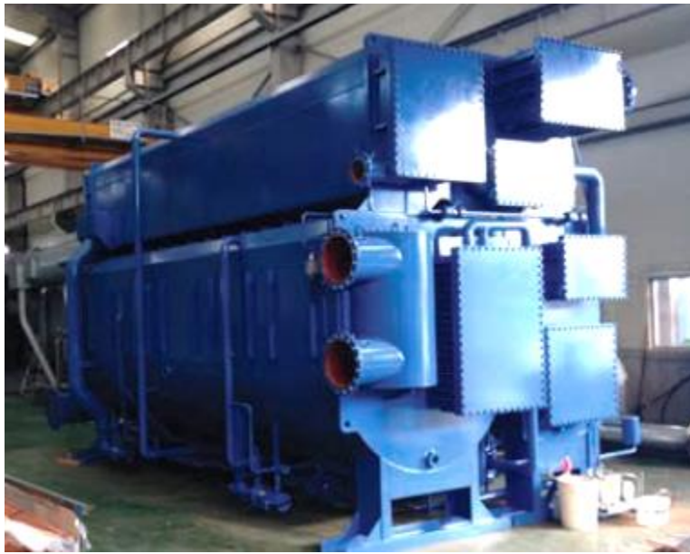
Figure 2-3: Maritime absorption chiller by Heinen & Hopman [43]
