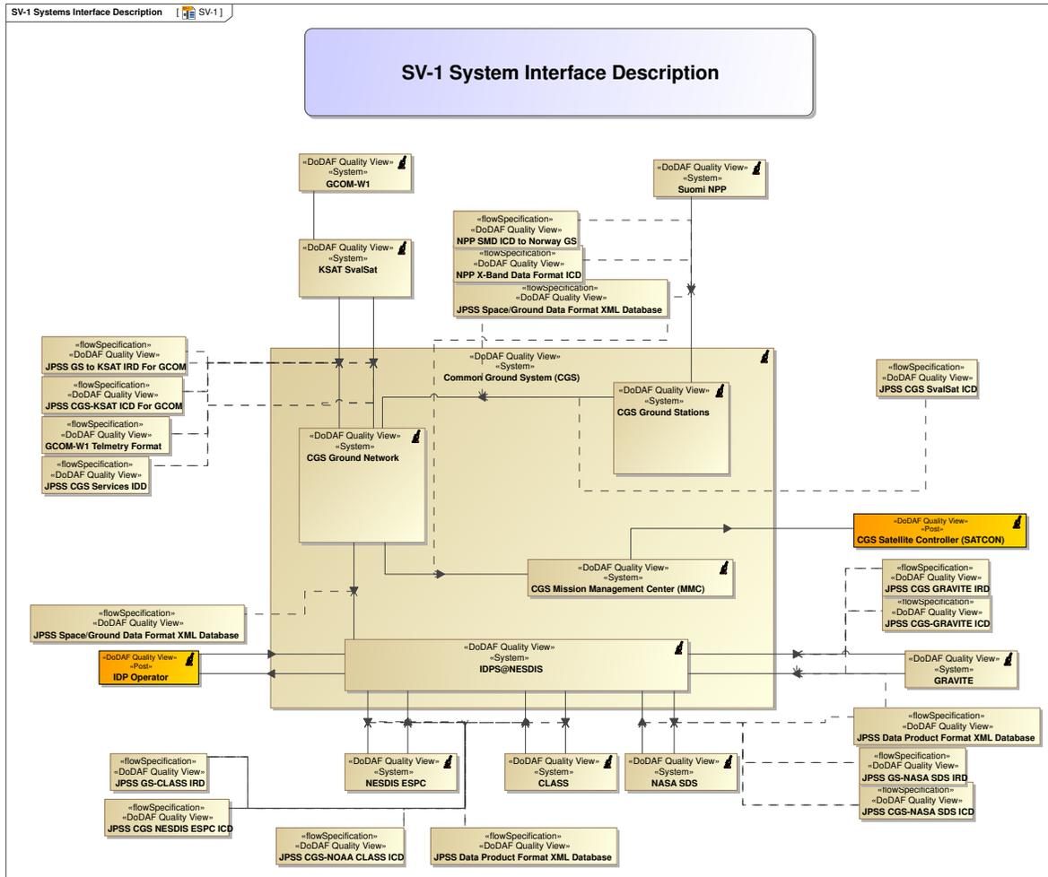
**Figure 4.5:** Joint Polar Satellite System (JPSS) DoDAF System Interface Description SV-1
