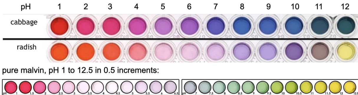
Figure 1.3: Anthocyanin extracts from cabbage and radish, and pure malvin, at a range of pH values. Extracts prepared by S. Thompson [15].
