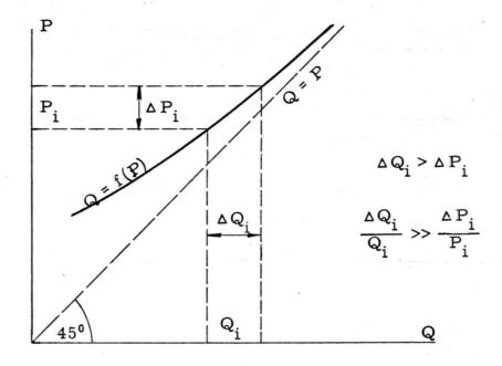
Fig. 1 General precipitation - runoff relationship for annual values, Q = f(P). An increase in annual precipitation represents a larger absolute or relative increase in runoff.
