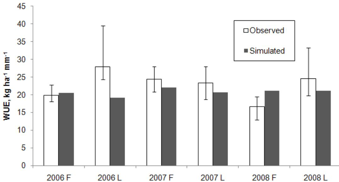
**Figure 2-6. Water use efficiency (WUE) for all treatments and years. F indicates full irrigation, and L indicates limited irrigation. Error bars indicate maximum and minimum observed values.**
