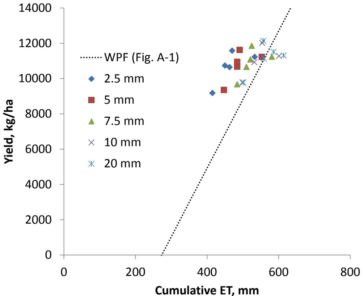
**Figure A-2. WPF simulations using hypothetical limited irrigation treatments. Dotted line taken from WPF line defined by Figure A-1. Treatment name in legend indicates weekly irrigation amount during the vegetative stage (mm). No water stress occurred during the reproductive stage for any treatment.**
