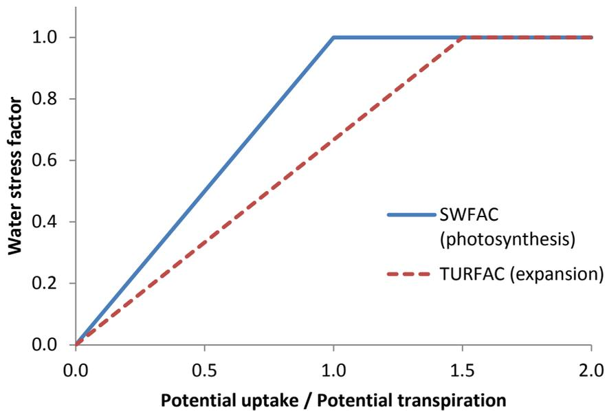
**Figure 4-2. Water stress factors used in DSSAT models (Ritchie, 1998 via Saseendran et al., 2008b).**
