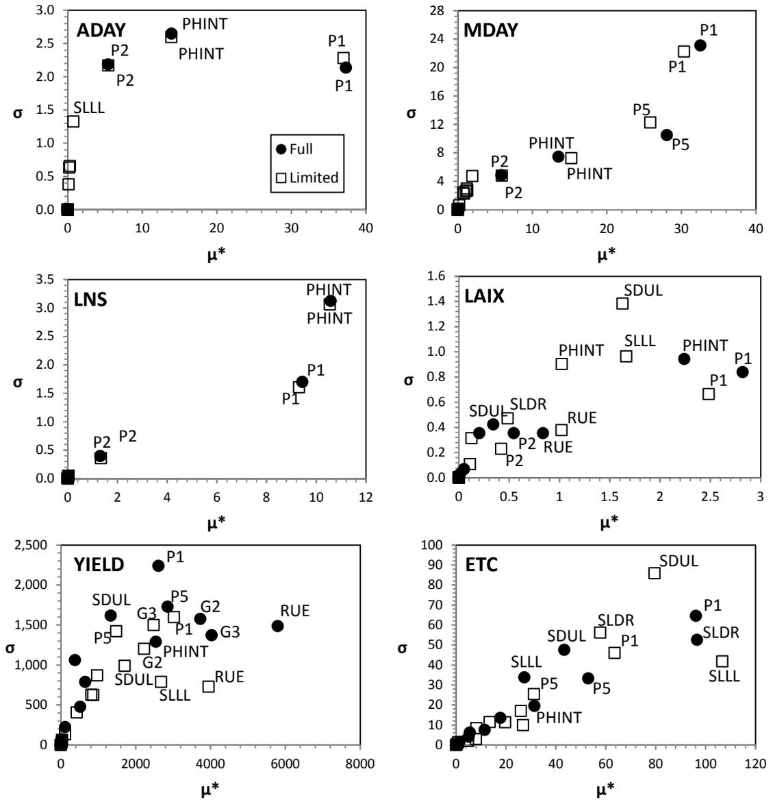
**Figure 3-1. Morris sensitivity analysis results shown in graphical form for all CERES-Maize output responses of interest. Filled circles indicate full irrigation treatment, open squares indicate limited irrigation treatment. Labels of the most important factors are shown.**
