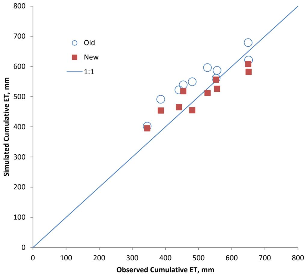
**Figure 4-11. Simulated vs. observed cumulative evapotranspiration (ET) for the original and new model.**
