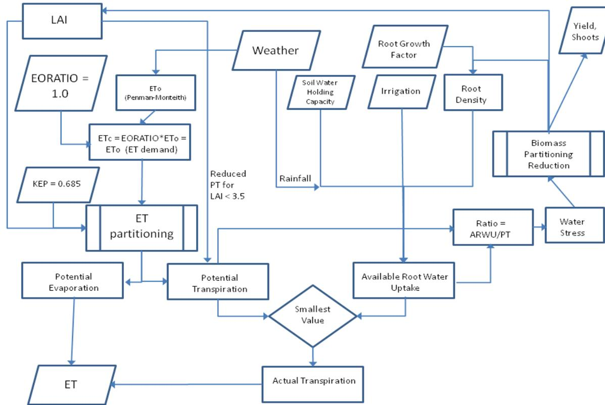
Figure 4-1. Logic of current ET calculation in CERES-Maize model.
