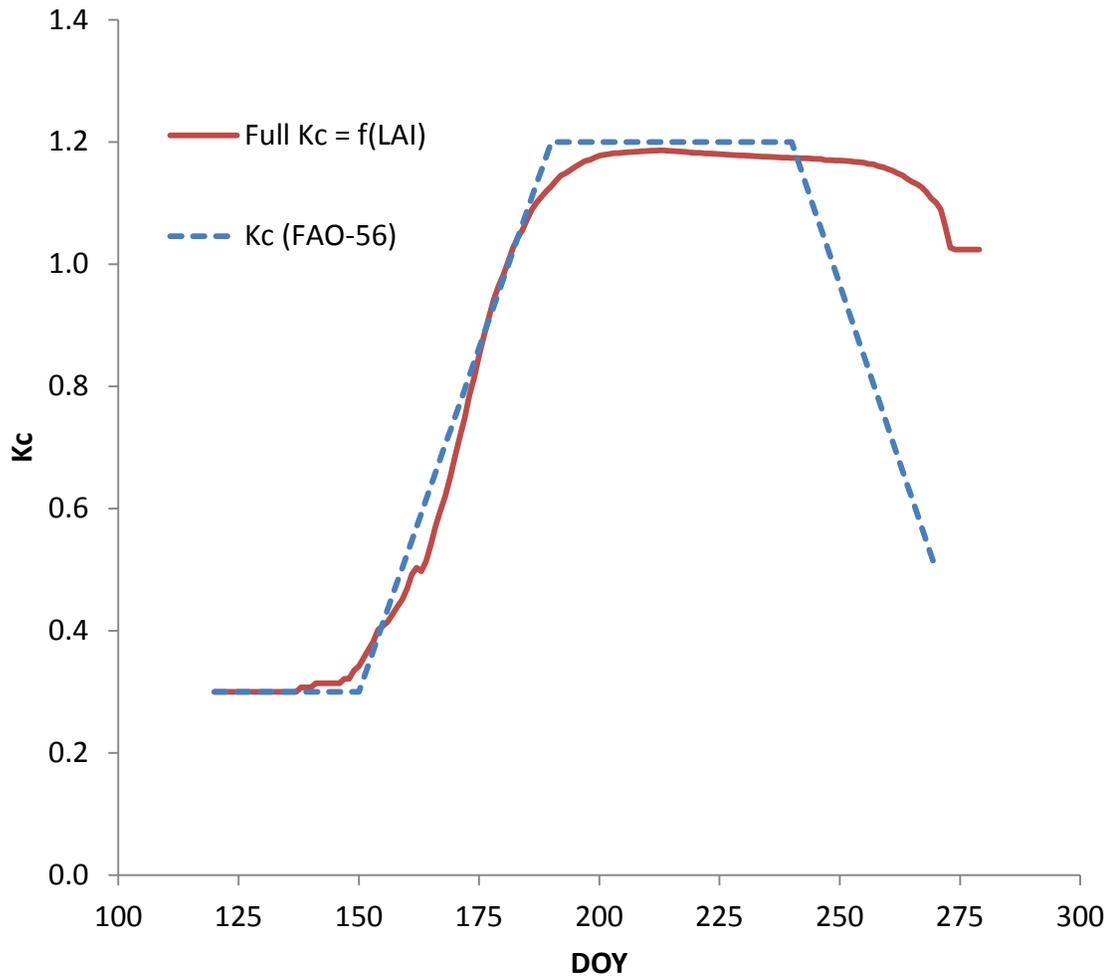
**Figure 4-8. Crop coefficient curve for potential ET in full irrigation treatment (2008) as a function of LAI, found by Eqn. 4-11. For comparison purposes, a crop coefficient curve from FAO-56 is also shown (Allen, 1998).**
