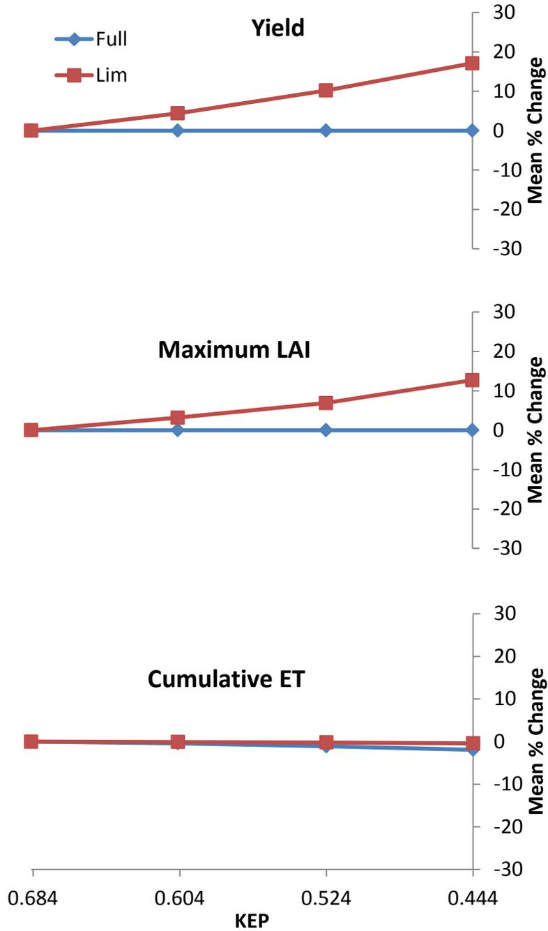
Figure 4-7. Local sensitivity of yield, maximum LAI, and cumulative ET to changes in KEP, for full and limited irrigation treatments. Vertical axis indicates change in output (%) from baseline (KEP = 0.685) averaged over five years simulated.
