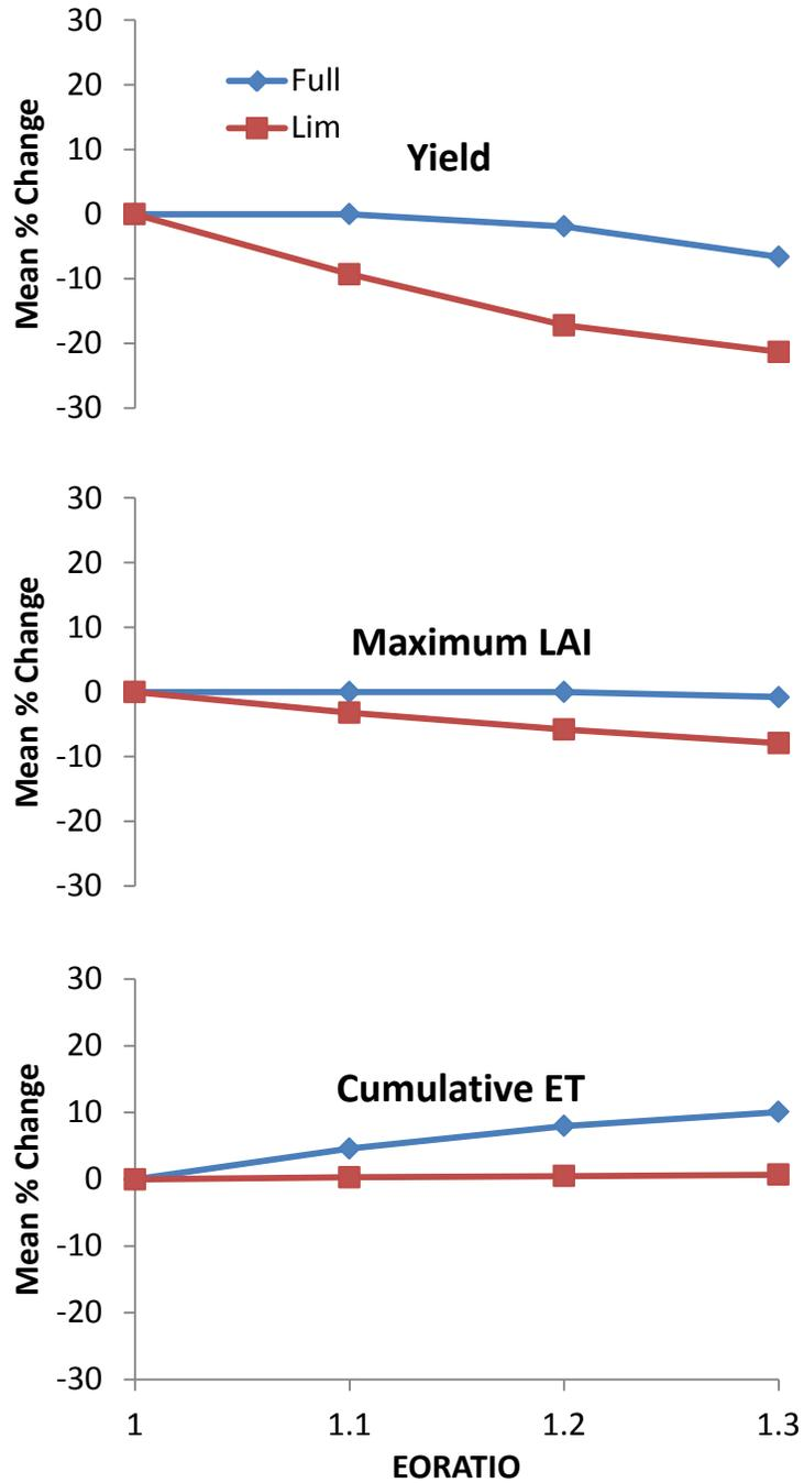
Figure 4-6. Local sensitivity of yield, maximum LAI, and cumulative ET to changes in EORATIO, for full and limited irrigation treatments. Vertical axis indicates change in output (%) from baseline (EORATIO = 1.0) averaged over five years simulated.
