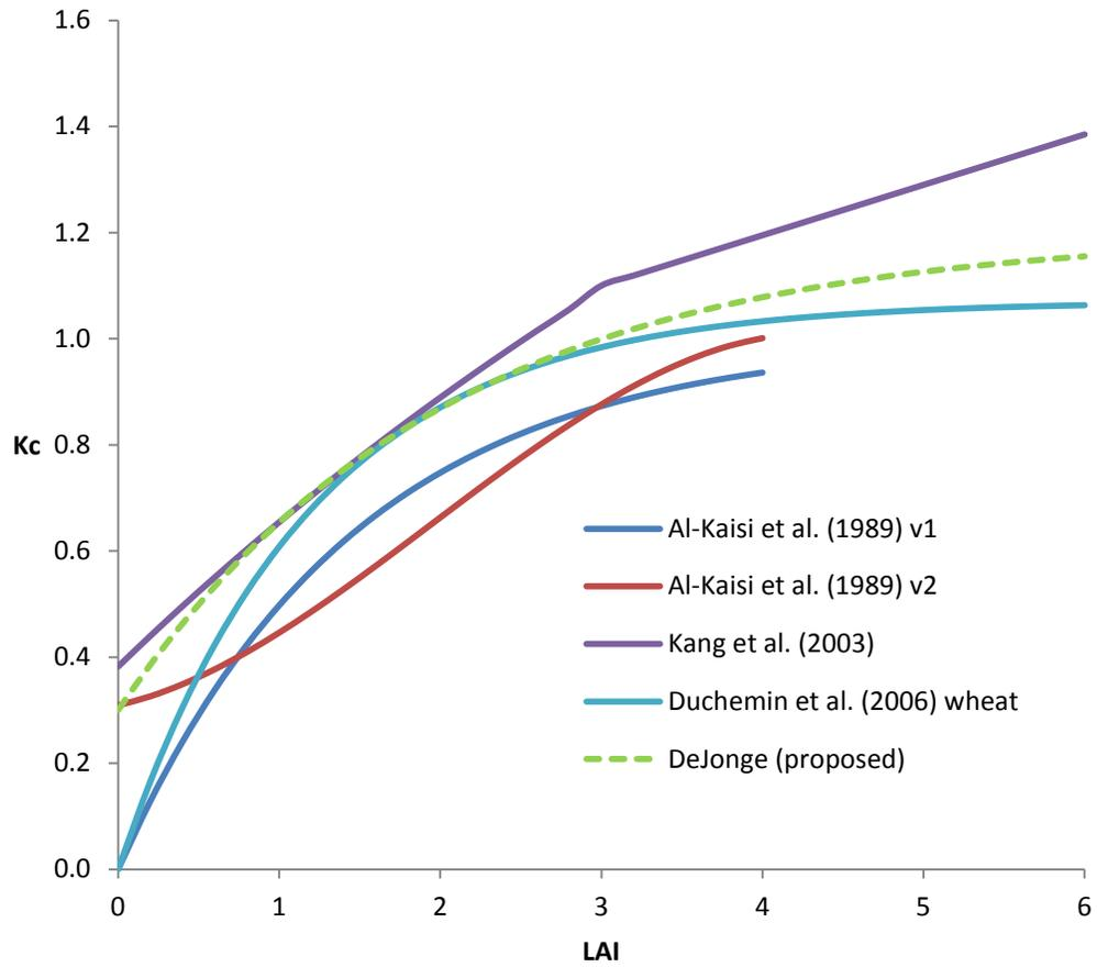
**Figure 4-4. Crop coefficient (Kc) versus leaf area index (LAI) relationships found in literature, and newly proposed function for this study.**
