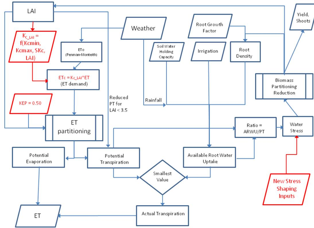
Figure 4-5. Logic of ET calculation in CERES-Maize model with model changes (in red).
