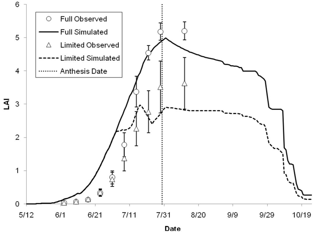
**Figure 2-3. Leaf area index (LAI) in 2008 for both irrigation treatments. Error bars on observed data indicate one standard deviation from the mean.**
