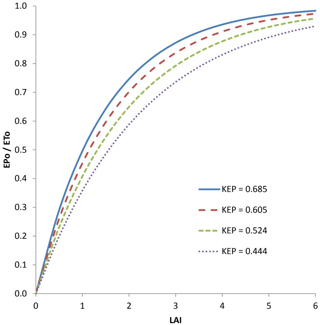
**Figure 4-3. Partitioning of potential plant transpiration as a fraction of potential ET, based on LAI, for varying KEP values.**
