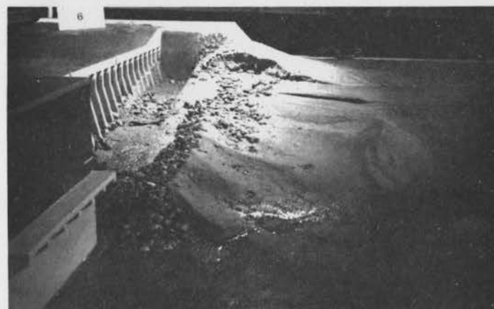
C Scour Conditions Downstream from Abutment
