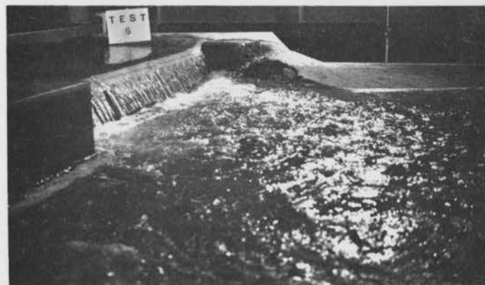
B Flow Conditions and Scour at North End of Abutment
