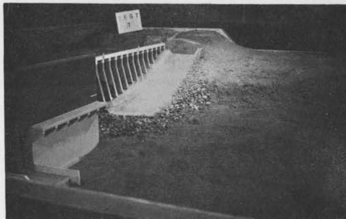
A Concrete-lined Channel and Riprap Armor, Before Test
