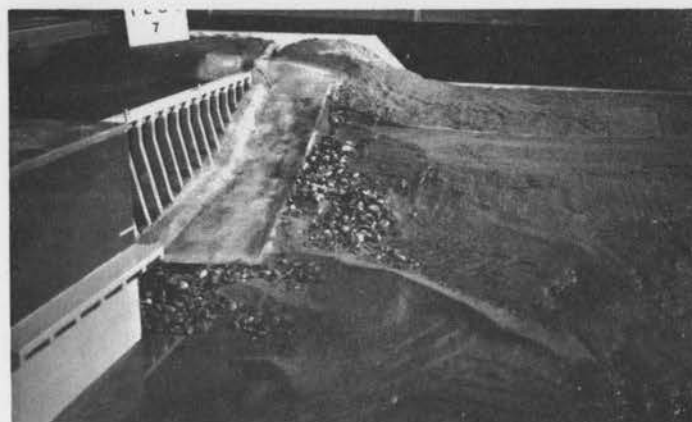
C Scour Conditions Downstream from Abutment Section
