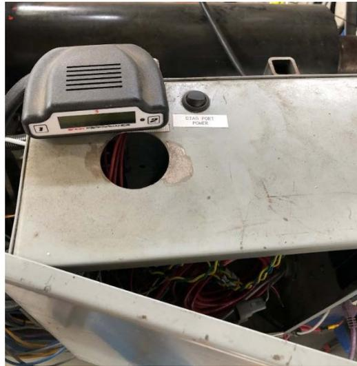
**Figure 62. Diagnostic Port Power Switch**
