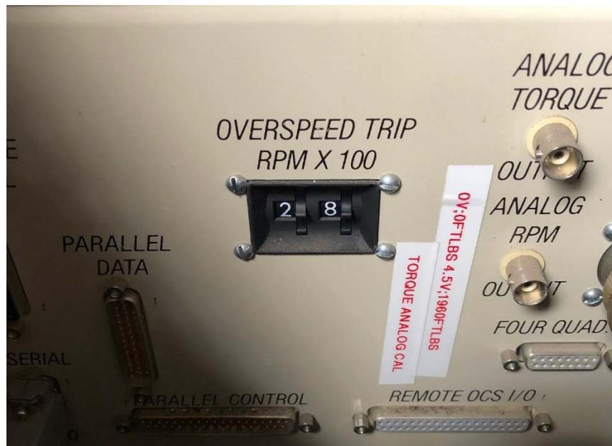
**Figure 45. Dynamometer Overspeed Protection**
