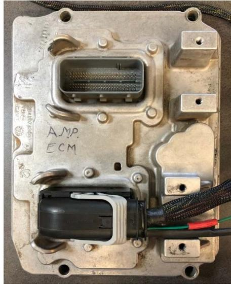
**Figure 40. CM2350 with Wiring Harness**
