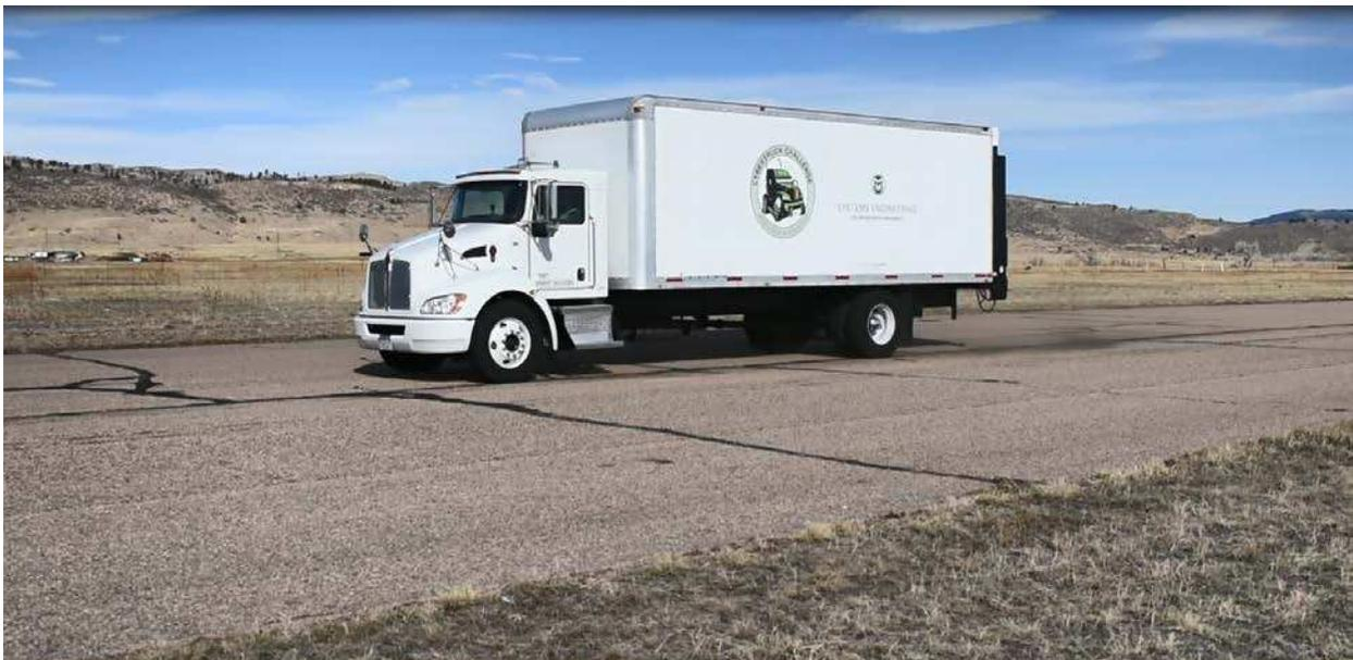
**Figure 5. Kenworth Conducting Hard Brake Maneuver at Christman Airfield**
