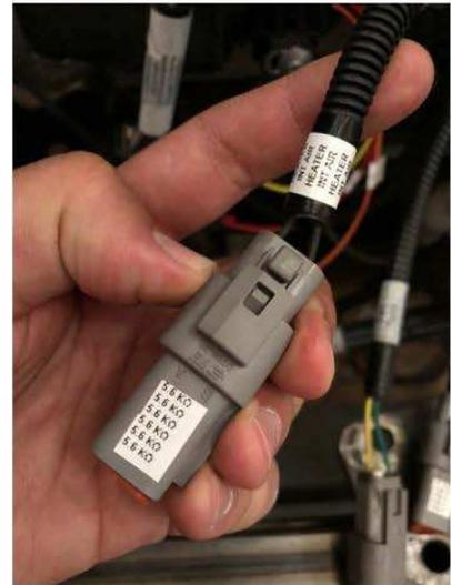
Intake Air Heater Sensor: 560  $\Omega$
