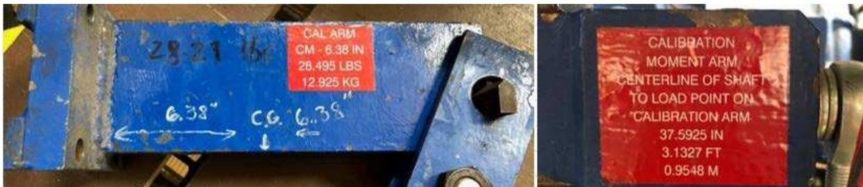
**Figure 30. Calibration Arm & Load Cell Moment Arm Dimensions**
