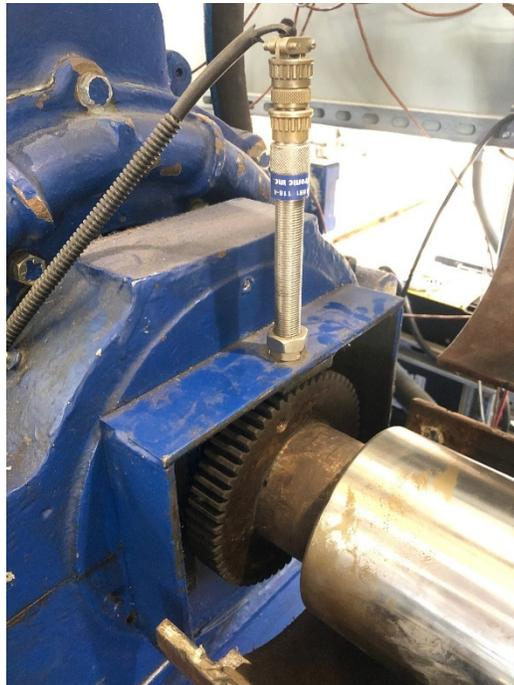
**Figure 32. Dynamometer Speed Pickup**
