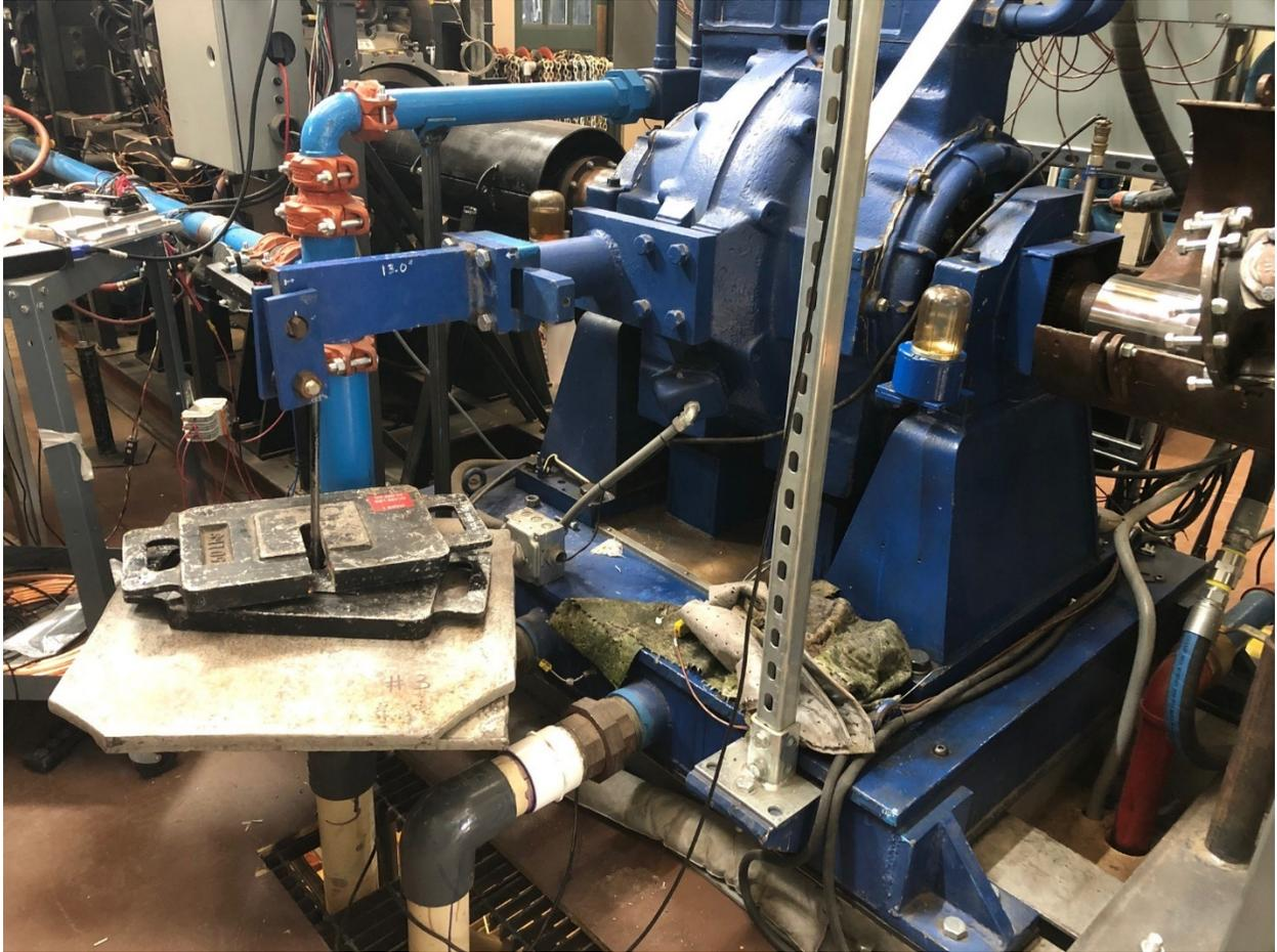
**Figure B-1. Dynamometer Load Cell Dead Weight Configuration**
