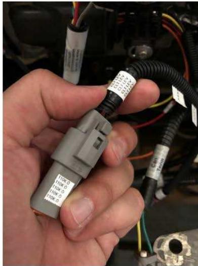
Coolant Level Sensor: 110 k $\Omega$
