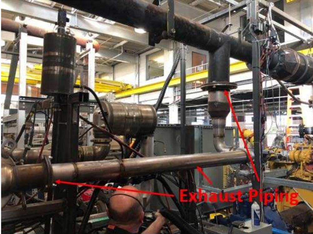
**Figure 13. Exhaust Pipe Fabricated**
