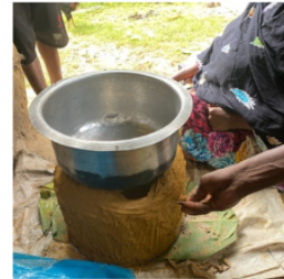
h) cut out hole for wood
