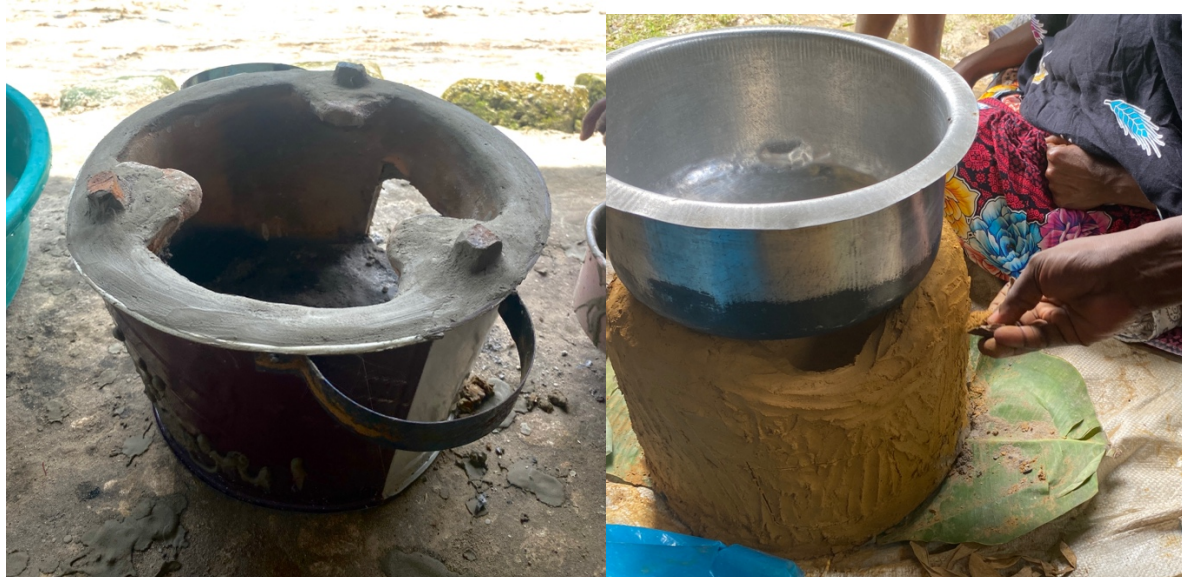
Figure 3. Image 1. Clay Efficient Cookstove (CES) with a metal casing. Image 2. CES being built from just clay before drying (DeGrandpre 2025).
