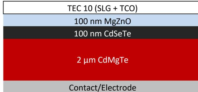
Figure 5.2.3: Device structure of a device containing the CdSeTe front layer. Not to scale.
