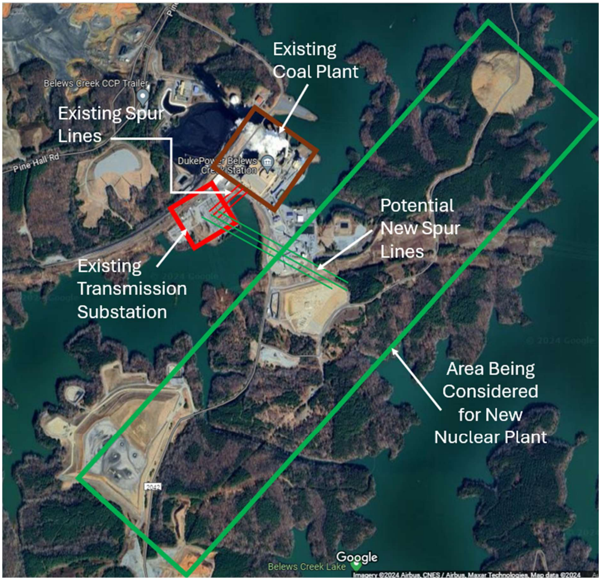
Figure 8. Aerial view of Belews Creek site showing existing coal plant location, location under consideration for new nuclear plant, existing transmission substation, existing spur lines, and potential new spur lines.
