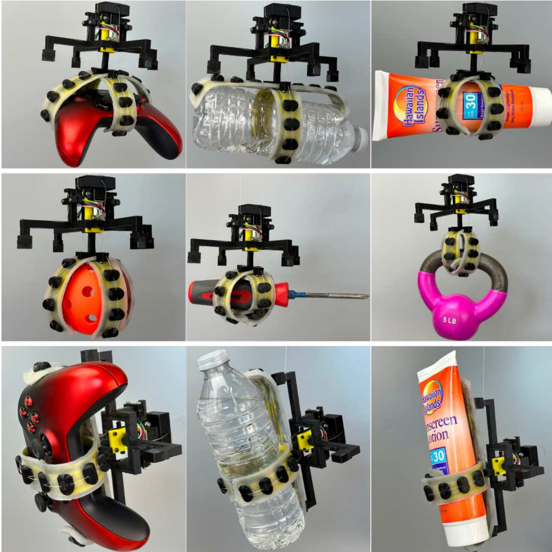
Figure 3.6: Object grasping performance for the silicone encased cross-shaped gripper in the horizontal axis where: (Top ) Horizontal grasping for the gripper for (left to right) a video game controller, half-full plastic water bottle, full sunscreen bottle; (Middle) Horizontal grasping for (left to right) a wiffle ball, screwdriver, and 5-pound kettlebell; (Bottom) Vertical grasping for the gripper with (left to right) a game controller, a full plastic water bottle, and a full sunscreen bottle.
