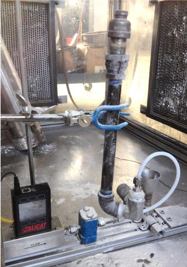
**Figure 6.7:** Second-generation fluidized bed burner
