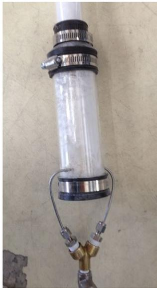
**Figure 6.5:** Fluidized bed burner with swirl
