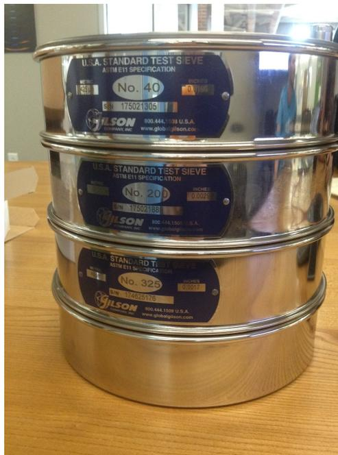
**Figure 11.1:** Sieve stack with coarsest mesh on top
