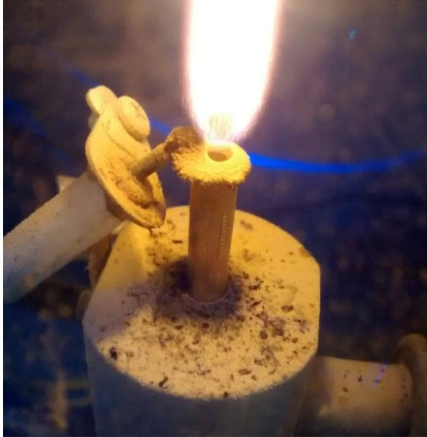
**Figure 9.1:** Lycopodium accumulating on Nano-Combustor nozzle and occluding bulk flow
