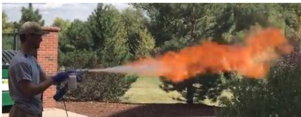
**Figure 5.4:** Powder Coating Gun with Cornstarch Flame
