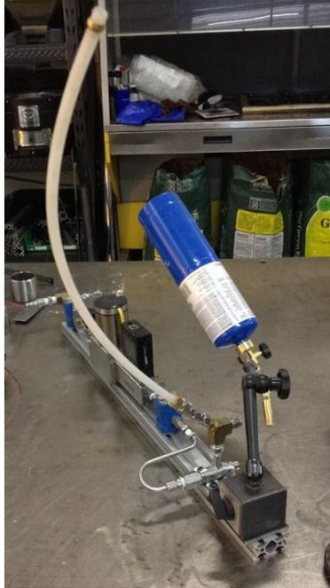
**Figure 5.12:** Venturi nozzle with pick-up tube
