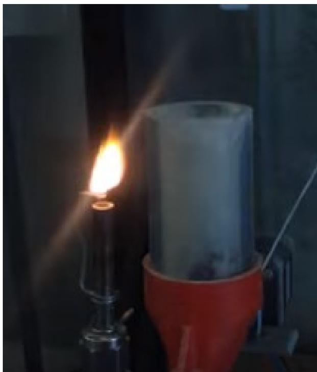
**Figure 8.3:** third-Gen Nano-Combustor, Rev. 2 flame, with flattened-wire flameholder
