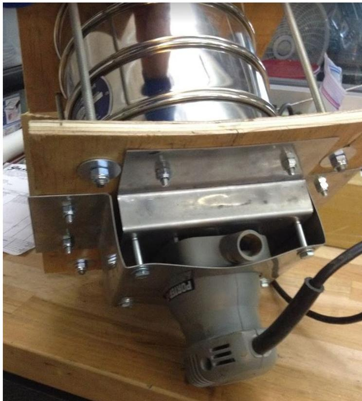
**Figure 11.2:** Sieve vibrator made out of a re-purposed palm-sander
