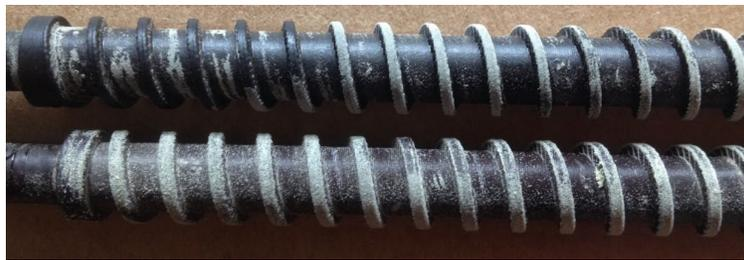
**Figure 8.10:** 3/8" OD 3/16" pitch augers. New auger on top with thinner flights
