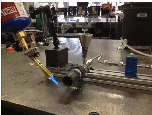
**Figure 5.7:** Venturi nozzle with hopper, nozzle, and torch
