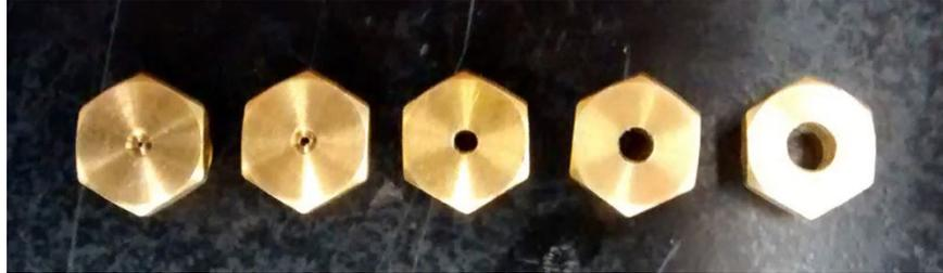
**Figure 10.4:** Lofting orifices ranging from 0.013" to 0.125" developed at MSR
