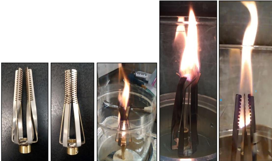
**Figure 10.1:** Examples of flameholder designs at MSR
