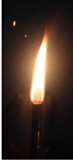
**Figure 8.5:** Third-Gen Nano-Combustor, Rev. 3 flame, with flared nozzle
