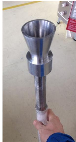
**Figure 6.6:** Fluidized burner with aluminum nozzle
