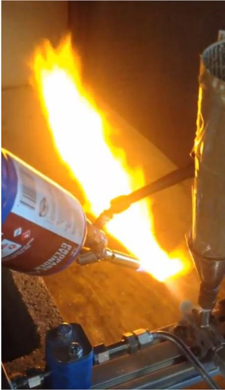
(a) Fox venturi flame lifting off without a diverging nozzle
