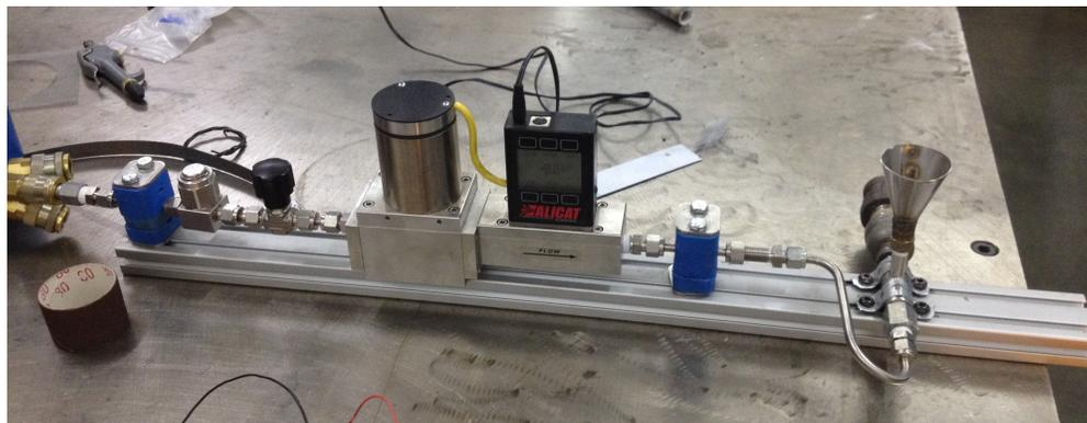
**Figure 5.8:** Venturi nozzle assembly
