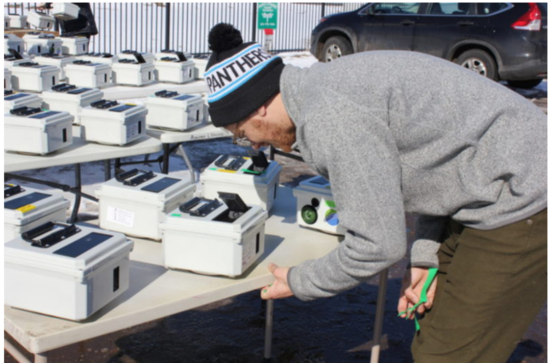
Lead author and alum Michael Cheeseman (M.S., '18; Ph.D., '22) inspects devices built by John Volckens's group that measure PM 2.5 particulate pollution.
