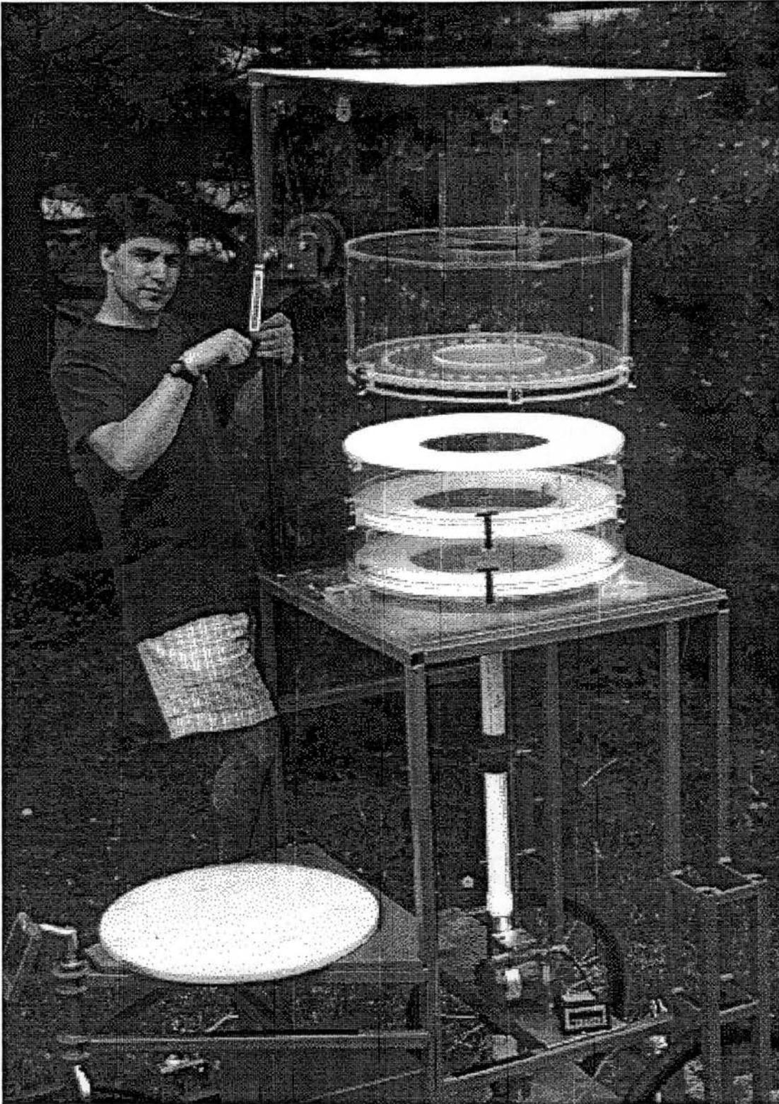
**Figure 2.4.** The IESL cloud impactor. The impaction plates are interchangeable with 50% lower size-cuts of 3, 4, 10, 12, 15, 20, and 30  $\mu\text{m}$ .
