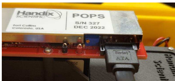
Figure 12. Gain adjustment on POPS.
