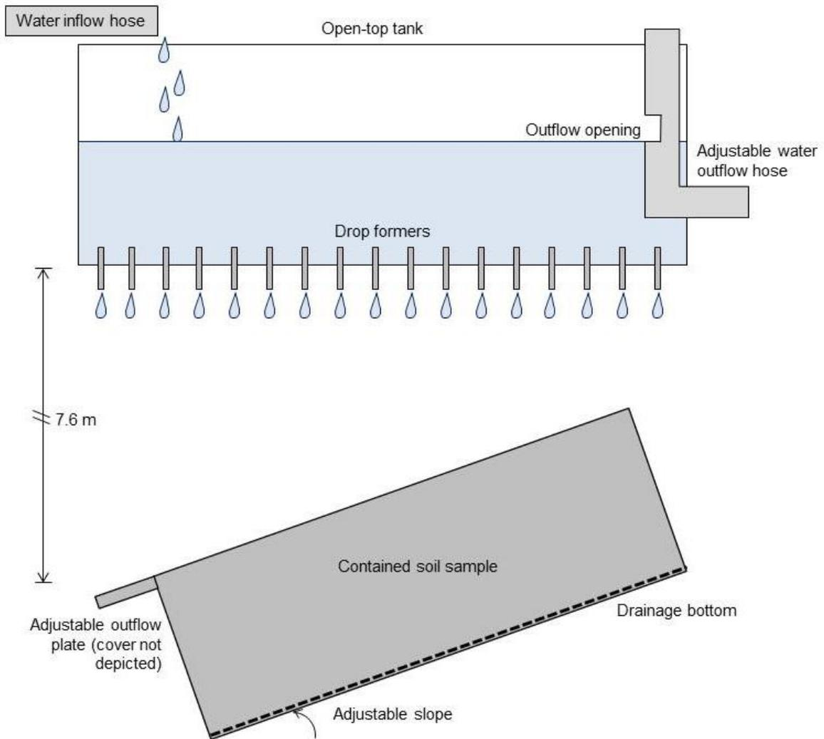
**Fig. 3.1.** Simplified schematic of the rainfall simulator (top) and soil container (bottom) used to conduct the slope-model experiments.
