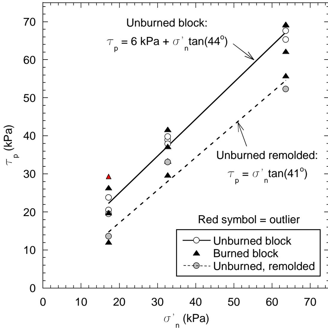
**Fig. 4.6.** Strength envelopes for undisturbed surface samples of unburned and burned soil and unburned, remolded soil using direct shear. The burned block outlier was due to an observed rock in the shear plane.
