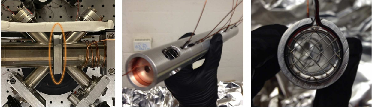
Figure 2.6: pictures of magnetic coil(a), copper disk(b) and extraction grid(c) [24]
