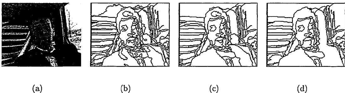
Figure 4.14: The segmentation resolutions with different \alpha values. (a) original car-phone image (frame 1), (b) \alpha = 7 , (c) \alpha = 13 and (d) \alpha = 17 .
