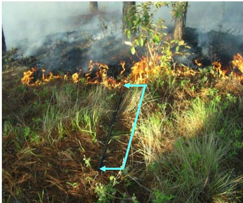
Figure 3.5. A direct method of measuring the rate of spread and of estimating flame height, when it is possible to work safely next to the flames. In this example, we utilized a meter-long metal tube, visible in the photograph to the left of the blue line, plus an ordinary stop watch. An estimate of the average flame length in this photo would be 10 centimeters.
