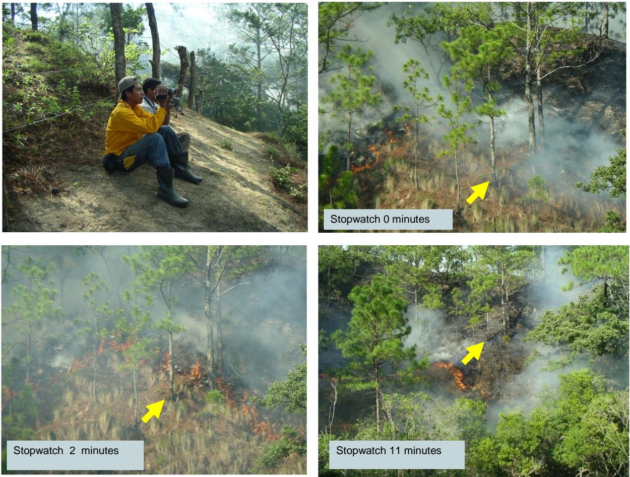
Figure 3.6. An indirect method for measuring the rate of spread, by analyzing video footage after the fire and measuring distances between trees or other points on the landscape. The location of the fire at two points in time, together with time passed, as indicated by either the timer inside the camera or a stopwatch, enable calculation of the fire's rate of spread.
