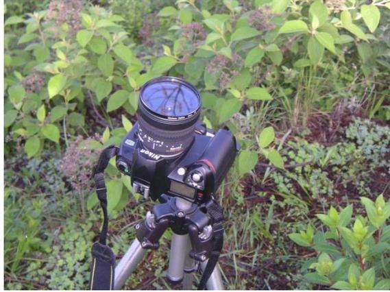
Figure 4.4a. Camera and fisheye lens used for hemispherical photography of the forest canopy.
