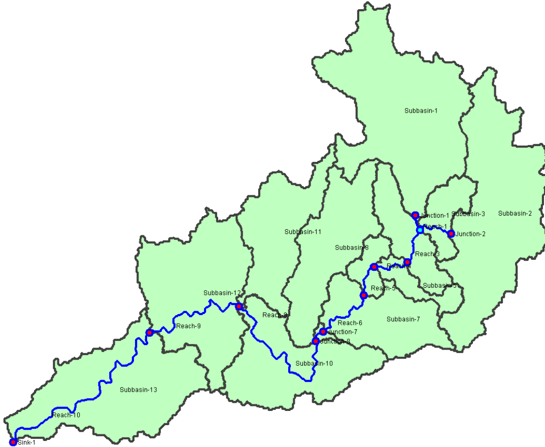
Figure 4.1: Disaggregation of basin in HEC-HMS
