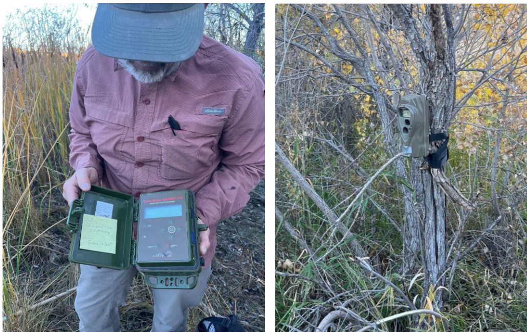
Figure 7. An acoustic monitor (left) and camera trap (right) being set up at the CSU-Foothills Campus.
