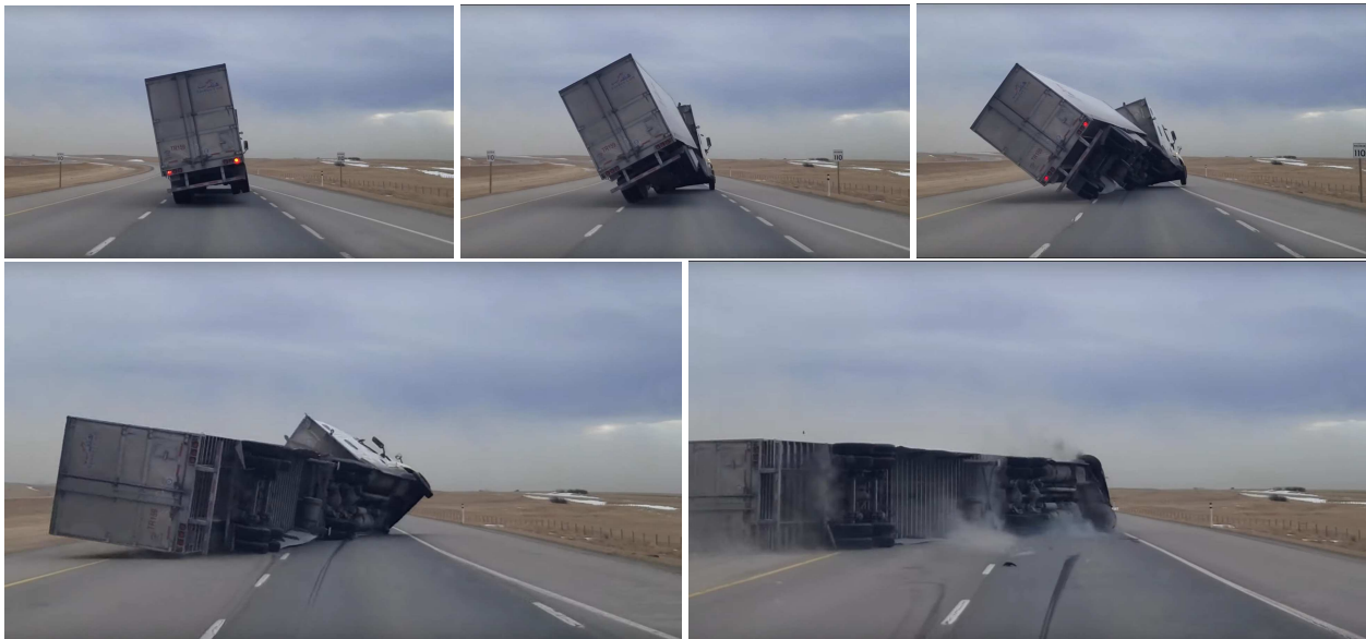
Figure 1.1: High sided vehicle overturning due to high crosswind. Images from The Weather Network.
