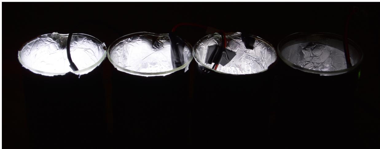
Figure 5.8. Picture of the relative light intensities used in this study, controlled by an LED dimmer. From left to right: 100%, 50%, 25%, 5% relative light intensity.
