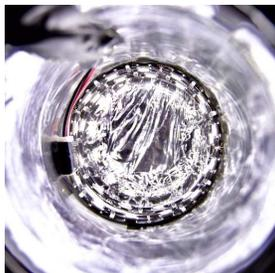
Figure 5.7 A picture of the photoreactor used for O-ATRP, constructed from a 400mL beaker lined with 45 cm of white LEDs.
