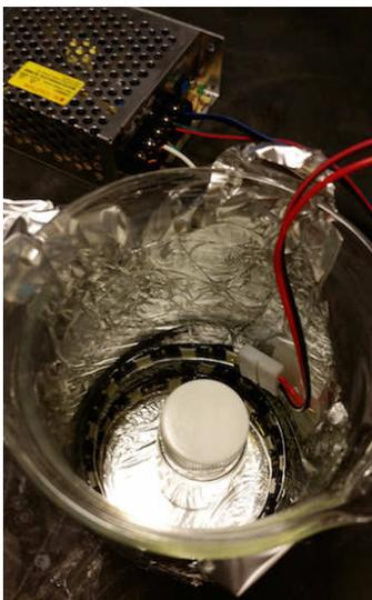
Figure 2.5. Photograph of the general reaction setup for polymerizations using LED irradiation.
