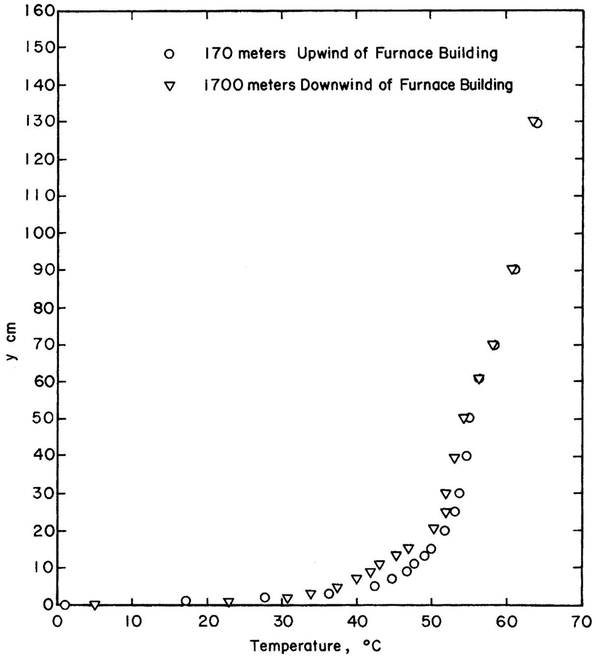
Figure 10. Vertical Temperature Profiles Measured in Wind Tunnel for Intermediate Stability Case
