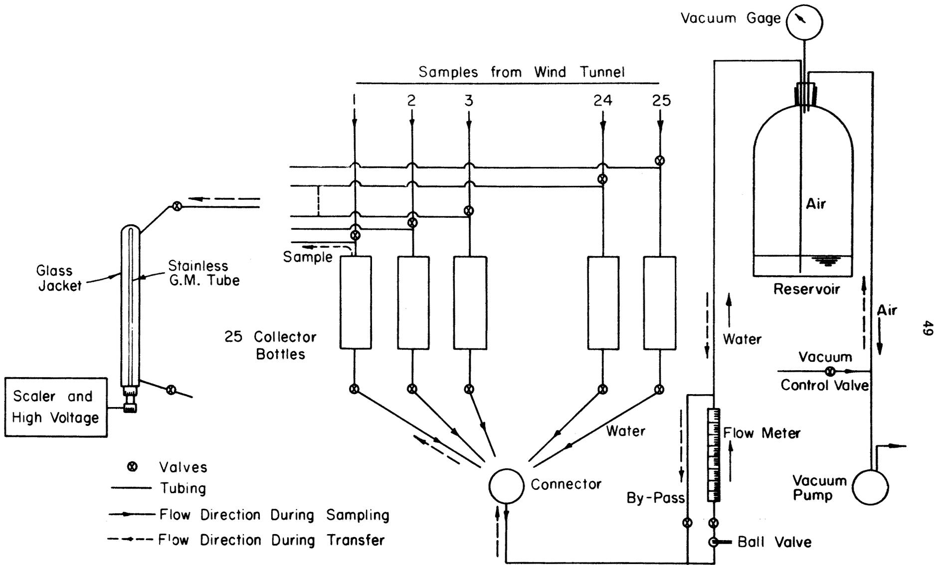
Figure 5b. Tracer-gas Sampling and Analysis System
