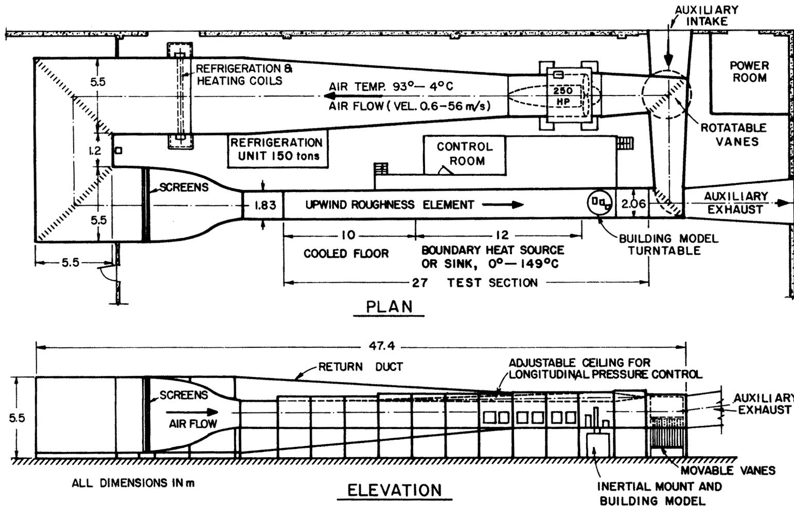
FIG. 1. METEOROLOGICAL WIND TUNNEL (Completed in 1963)
