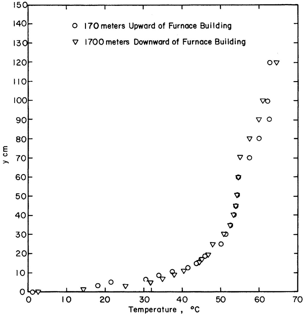
Figure 9. Vertical Temperature Profiles Measured in Wind Tunnel for Maximum Stability Case
