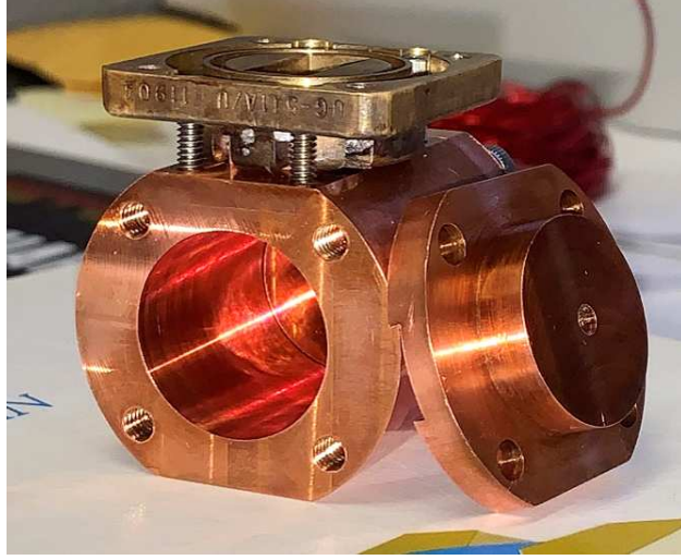
Figure 1.3: A cylindrical microwave resonant cavity open at one end. The cavity couples to a Ku-band rectangular waveguide.
