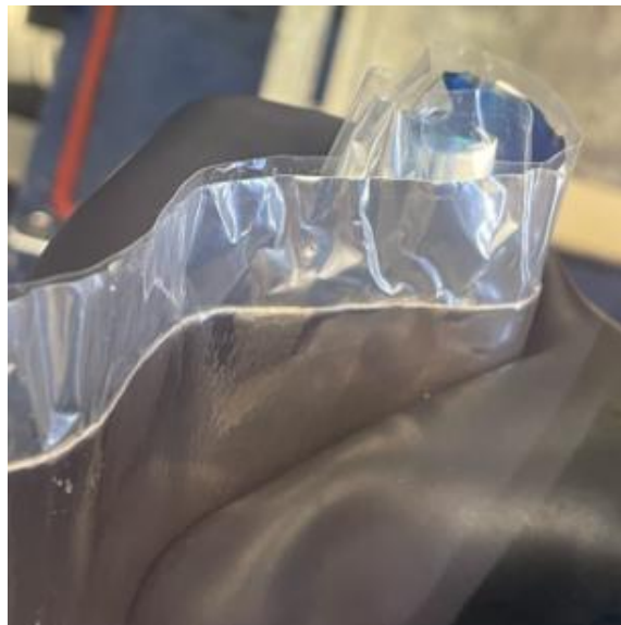
Figure 3-1: Close image of the composite sodium material. The grey material closest in the forefront of the image is the sodium, and shiny silver material in the back is the aluminum current collector. Between the two is a white material serving as a binder, that is unidentified from by manufacturer.
