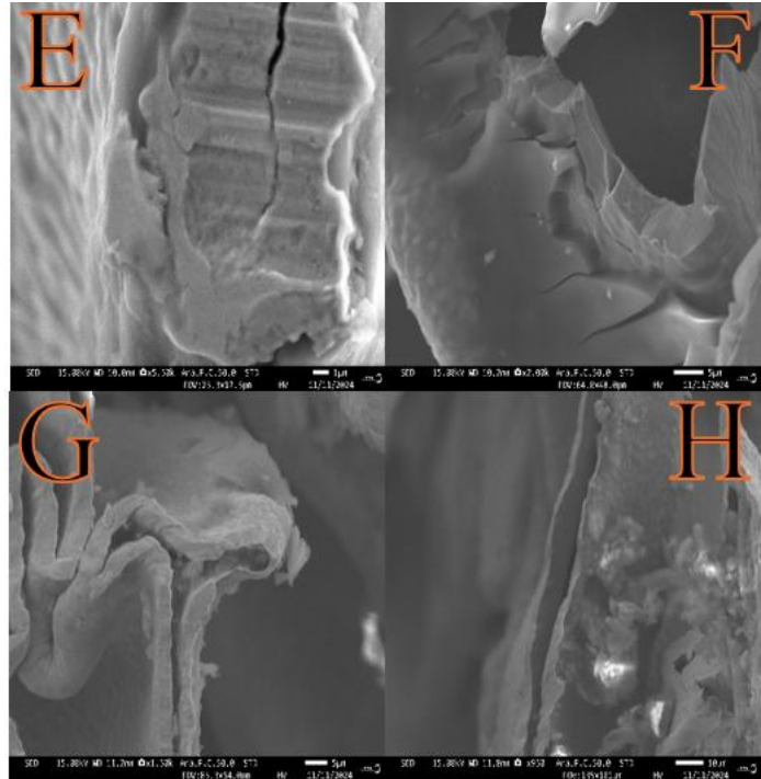
Figure 2-6: SEM images of cPAN from 0.5M PAN solution. TOP- E/F PAN 1 sample. Bottom- G/H PAN 2 sample.
