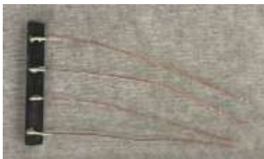
Figure 3.02 Electrical Conductivity PPMS Sample
