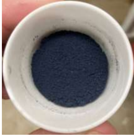
Figure 4.01 Strontium Vanadate Powder (SVOP) Post Furnace Heating in 5:95 H 2 :N 2 Environment
