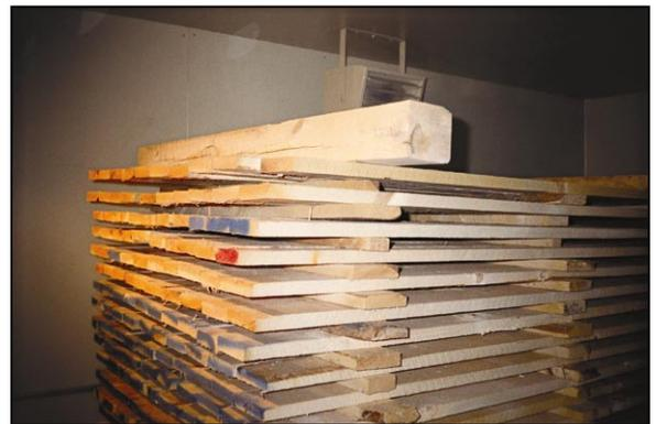
***Above: Figure 3. Ponderosa pine lumber being dried in a small de-humidification dry kiln in Lewis, Colorado.***
