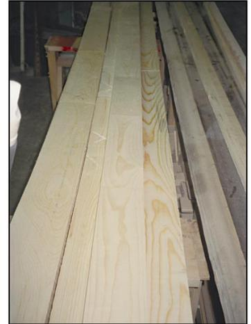
***Figure 2. - Clear (no knots), finger-jointed and edge glued ponderosa pine.***
