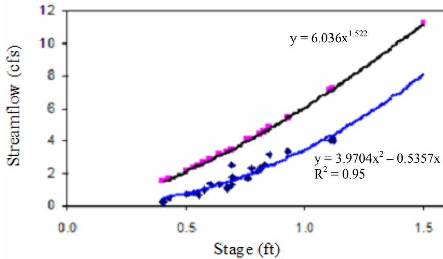
**Figure 5.2.** New stage-discharge relationship (bottom) derived from field measurements compared to precalibrated flume stage-discharge relationship (top).
