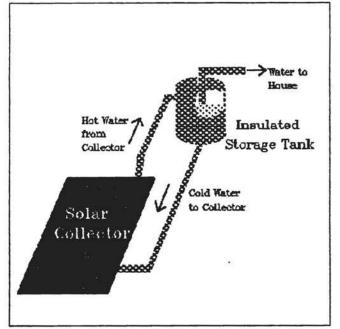
suited to preheat water. As shown in the figure on the left, the water is
