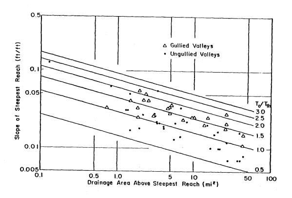
Figure 4 Plot of data from Fig. 1 showing values of Relative Shear Stress Indicator (from Begin and Schumm, 1979).
