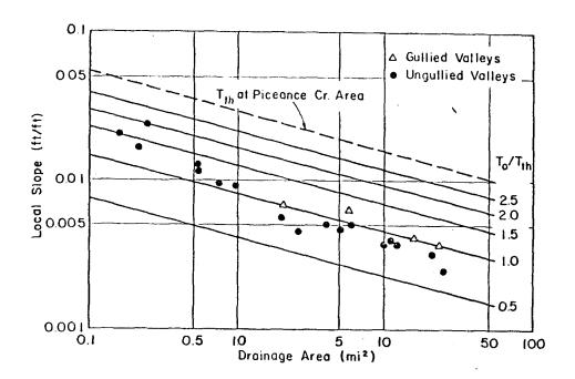
Figure 6 Drainage area valley-slope plot showing Relative Shear Stress Indicator for Brice's Mebraska channels (from Begin and Schumm, 1979).
