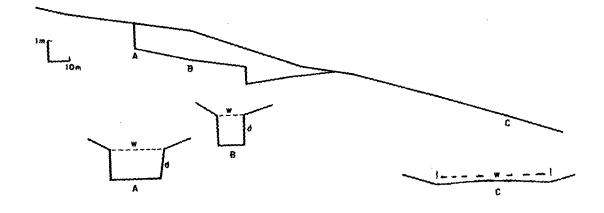
Figure 11 Longitudinal profile of valley and cross sections showing effect of valley floor slope and width on gully location.
