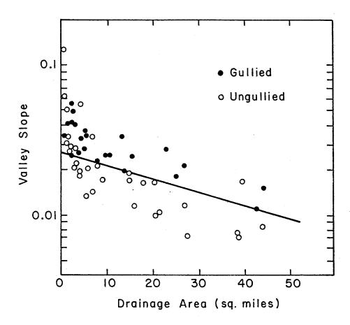
Figure 1 Relation between critical valley-floor slope and drainage area for small drainage basins, Piceance Creek area, western Colorado (from Patton and Schumm, 1975).
