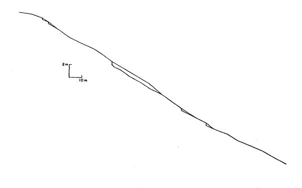
Figure 10 Longitudinal profile of valley showing multiple convexities and gullies.
