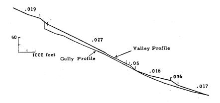
Figure 2 Longitudinal profile of Greasewood Creek, western Colorado. Note irregular valley-floor profile and discontinuous gullies cut below valley floor.
