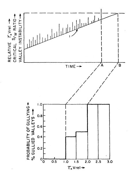
Figure 15 Change of valley - floor stability with time, as related to the probability of gullying for increased values of Relative Stream Power. See text for discussion of these relationships.
