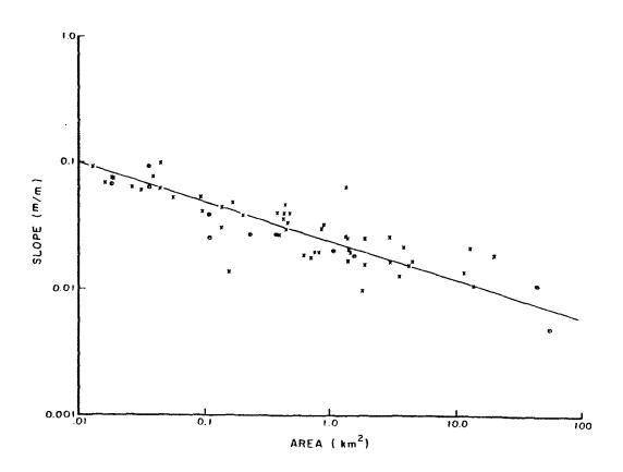
Figure 12 Plot of drainage area and critical valley slope, Chalk Bluffs area. x = gullied, o = ungullied valleys.
