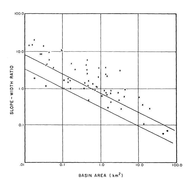
Figure 13 Plot of valley-slope - width ratio against drainage area.
