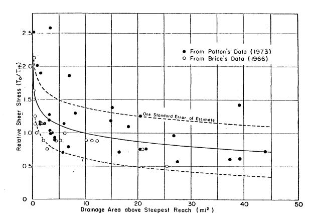
Figure 5 Relation between drainage area and Relative Shear Stress Indicator for ungullied valleys. The curve is a least-square semi-log fit; the correlation coefficient is 0.5, significant at a 0.01 level (from Begin and Schumm, 1979).
