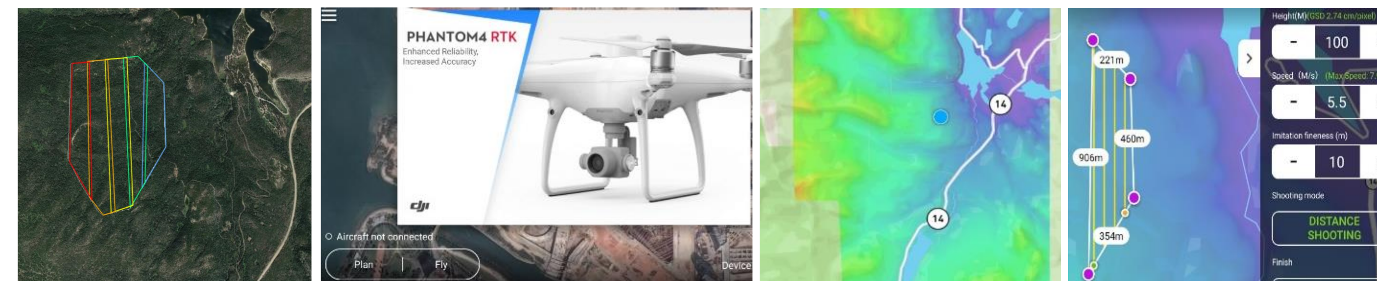
Figure 1. Google Earth KML files of the Blue Lake study site were imported with a DEM into the RTK controller for flight planning.
