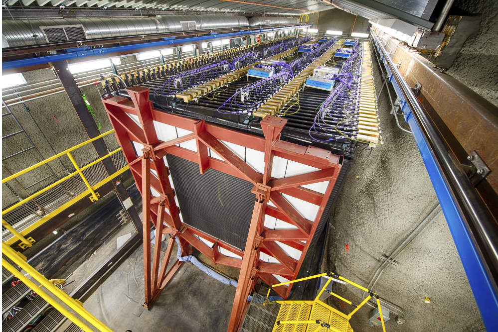
FIGURE 3.10. Photograph of the ND at Fermilab. The detector dimensions are 4.2\text{ m} \times 4.2\text{ m} \times 15.8\text{ m} . The camera is pointed toward the beam direction.
