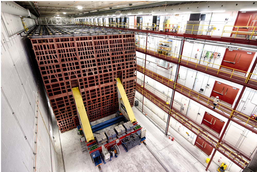
FIGURE 3.11. Photograph of the FD in Ash River, Minnesota. The detector dimensions are 15.6\text{ m} \times 15.6\text{ m} \times 63.0\text{ m} . The camera is pointed toward the beam direction.
