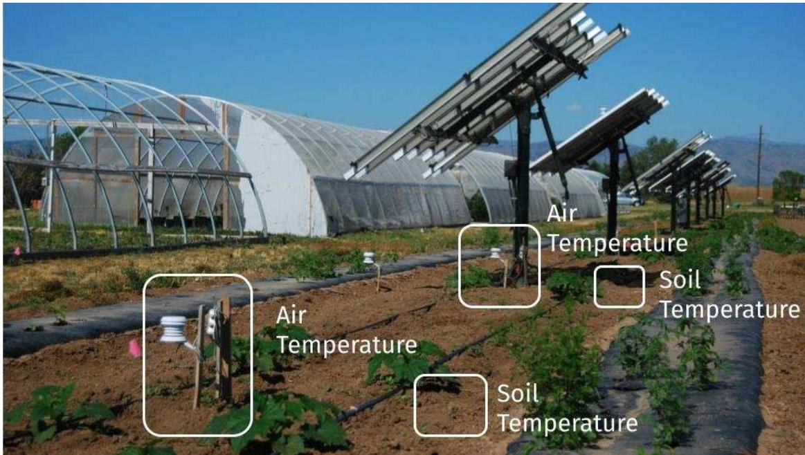
Figure 27: Air and soil temperature data collection points.
