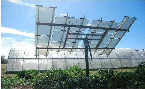
**Figure 11.** Experimental APV system with semi-transparent CdTe panels. Panels have 40% transparency.
