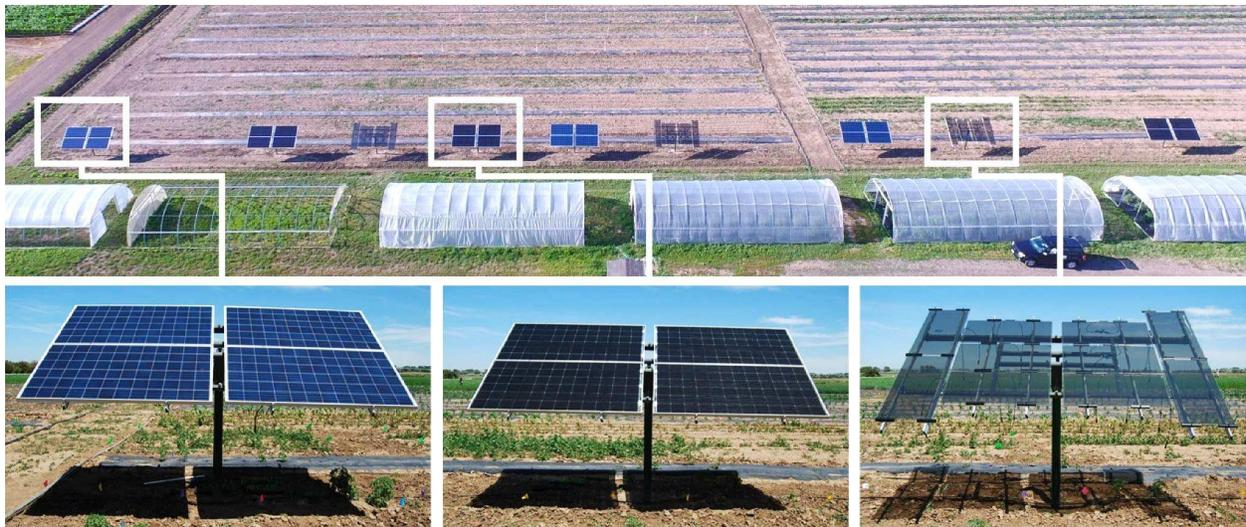
*Figure 24: Monofacial polycrystalline module (0% transparent), Bifacial monocrystalline module (~5% transparent), Cadmium telluride (CdTe) thin-film module (40% transparent)*
