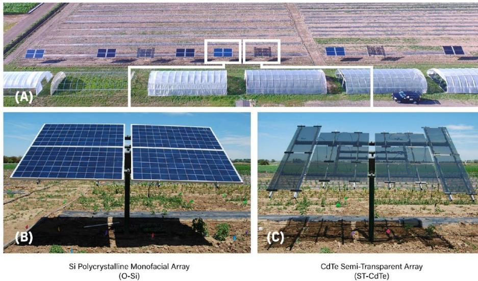
**Figure 12.** ARDEC site overview (A) Replicated AV test plots at CSU's ARDEC South location. (B) Opaque silicon (O-Si). (C) Semi-transparent CdTe (ST-CdTe).
