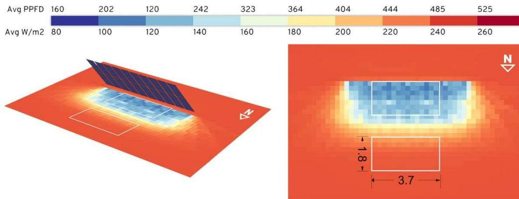
Figure 20: Analysis of average irradiance (perspective view, plan view, and legend) from July through October using SPADE Agrivoltaic Design Tool. Each white rectangle delineates the 3.7 m by 1.8 m full sun and shade treatment areas.
