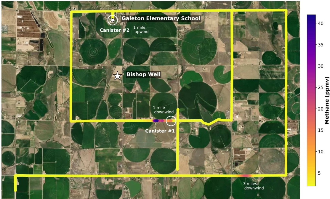
Figure 4.1: CH 4 concentration map from the drive on April 8, 2025 during the blowout at Bishop Well [40.5052°N, -104.5853°W] in Galeton, CO. The locations of the wellpad (white star), Galeton Elementary School (white filled circle), and canister samples (white hollow circles) shown on the map. The canister sample numbers from Table 1 and the distances from the wellpad are also annotated. The methane colorbar ranges from 1.9-41 ppmv.
