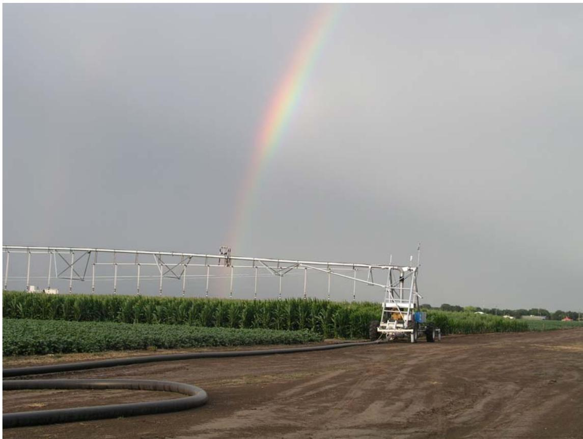
***Corn research plots being irrigated with a lateral move sprinkler irrigation system at Kansas State University.***
