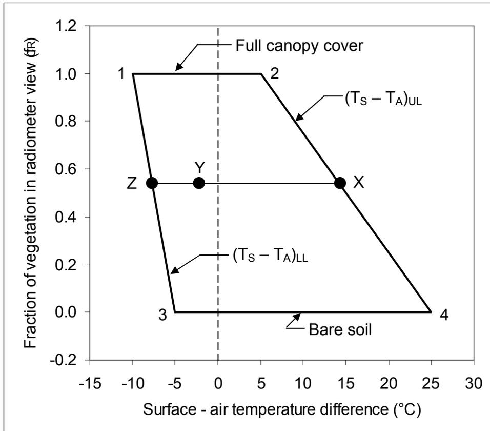
Figure 2. Water Deficit Index (WDI), defined as  $WDI = YZ / XZ$ . Point 1 is non water stressed full canopy, 2 is completely water stressed canopy, 3 is wet bare soil, and 4 is dry bare soil, and the lower and upper temperature limits are  $(T_S - T_A)_{LL}$  and  $(T_S - T_A)_{UL}$ , respectively (Moran et al., 1994).
