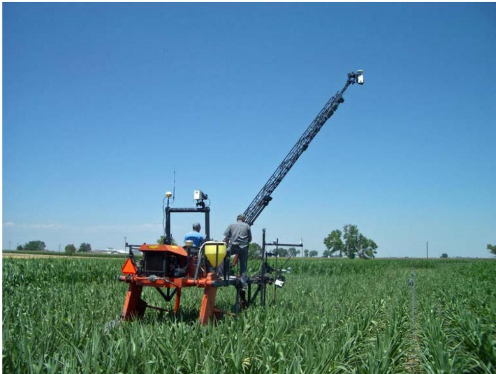
**Figure 2. High Boy reflectance tractor measuring canopy reflectance and temperature.**
