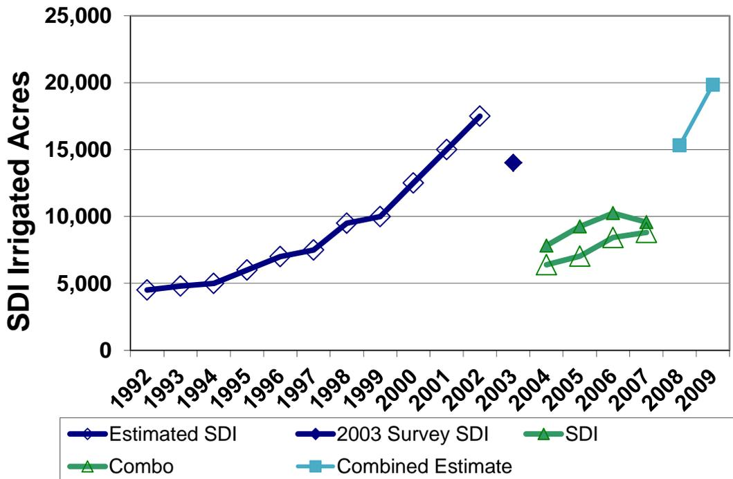
Figure 3. Increase in subsurface drip irrigation systems in Kansas. The abrupt changes in SDI area are due to survey and reporting methods and not due to abandonment of SDI systems. SDI has been increasing steadily in Kansas.
