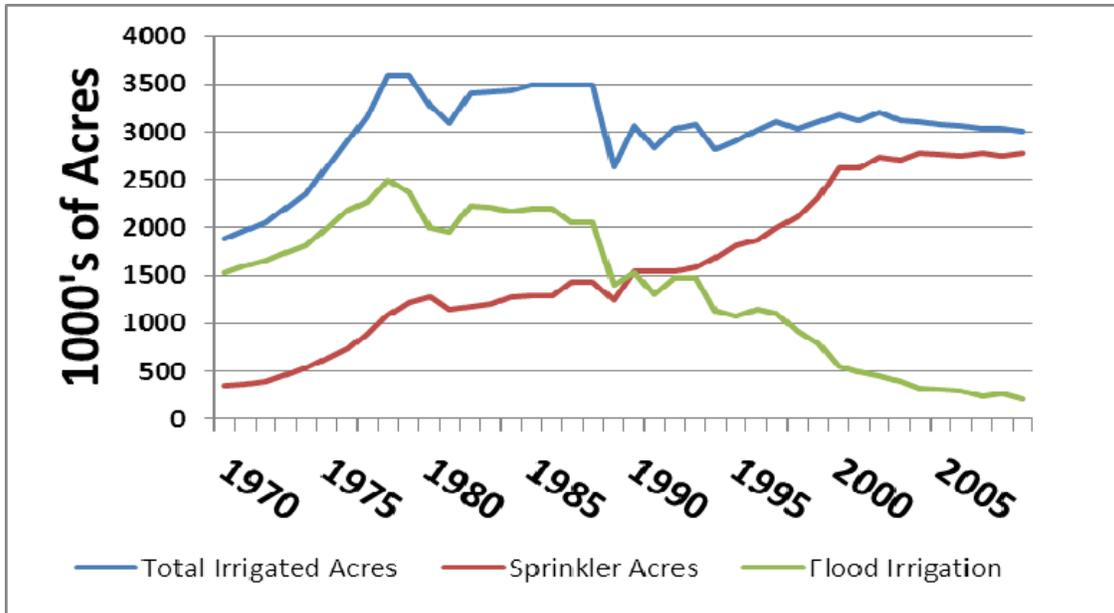
Figure 2. Progression of total irrigated land area, sprinkler systems, and flood Irrigation system Kansas.
