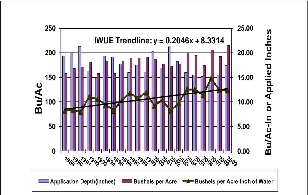
Figure 11. Corn yield, irrigation application depth, and irrigation water use efficiency trends for Southwest Kansas.
