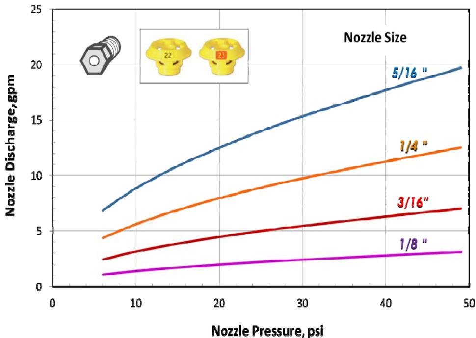
Figure 1. Performance of nozzles used in sprinkler devices
