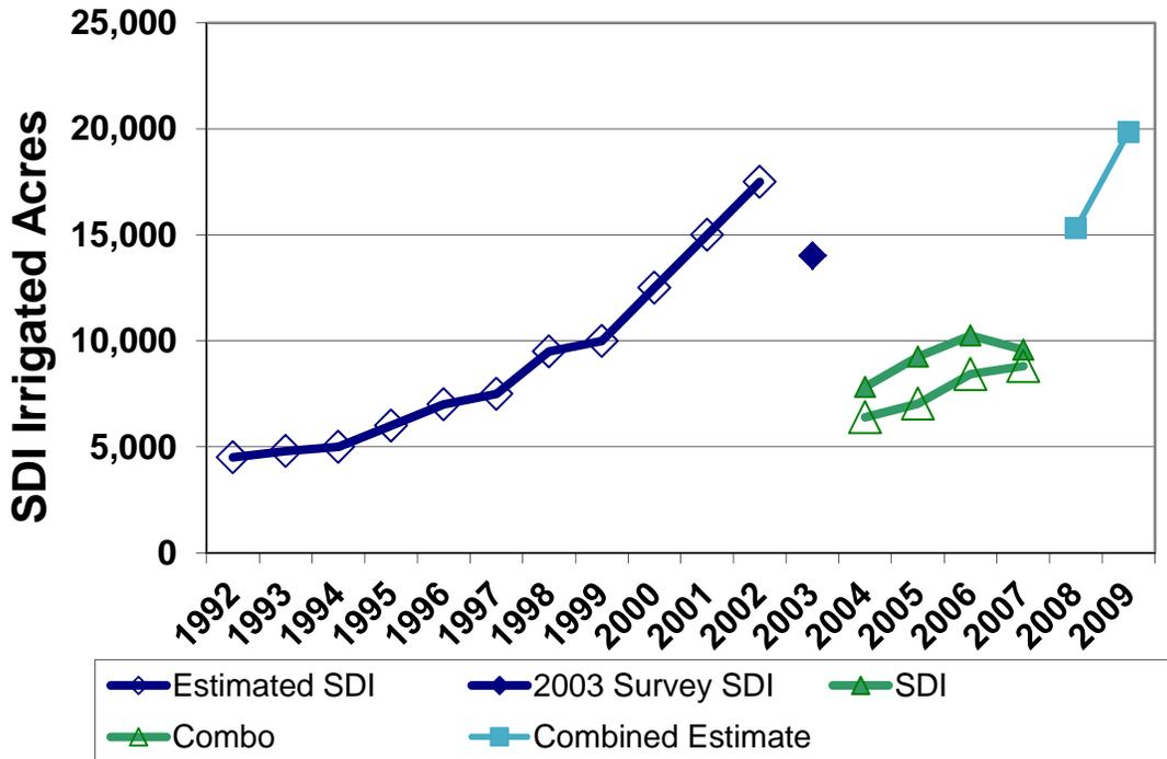
Figure 3. Increase in subsurface drip irrigation systems in Kansas. The abrupt changes in SDI area are due to survey and reporting methods and not due to abandonment of SDI systems. SDI has been increasing steadily in Kansas.
