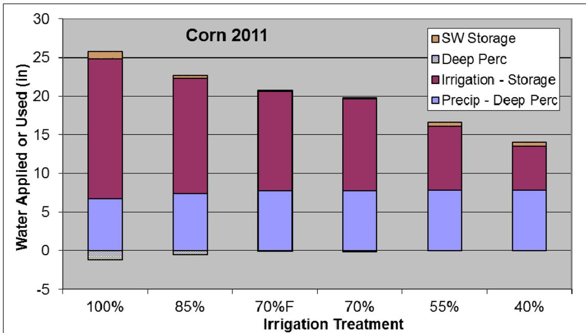
**Figure 3. Water balance for the 2011 corn crop showing precipitation, irrigation, and seasonal soil water storage changes. Bars below zero represent deep percolation losses.**
