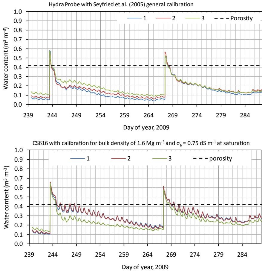
Figure 3. Hydra Probe water contents using Seyfried et al. (2005) general calibration (top); and CS616 water contents from calibration for sandy clay loam,  $\rho_b$  of  $1.6 \text{ Mg m}^{-3}$  and  $\sigma_a = 0.75 \text{ dS m}^{-1}$  at saturation (bottom) for the first two flooding and dry down periods, in Texas.
