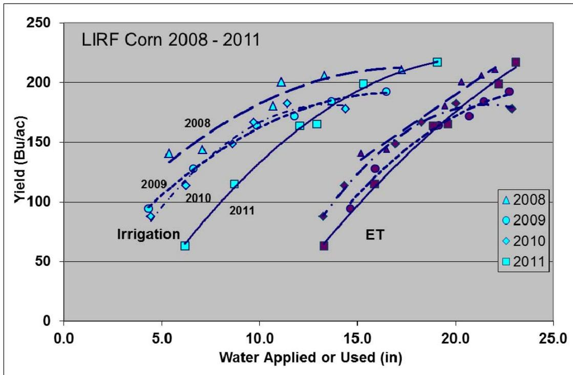
**Figure 6. Water production functions for 2008 - 2011 corn at LIRF. Left curves are yield vs. irrigation water applied; right curves are yield vs ET.**
