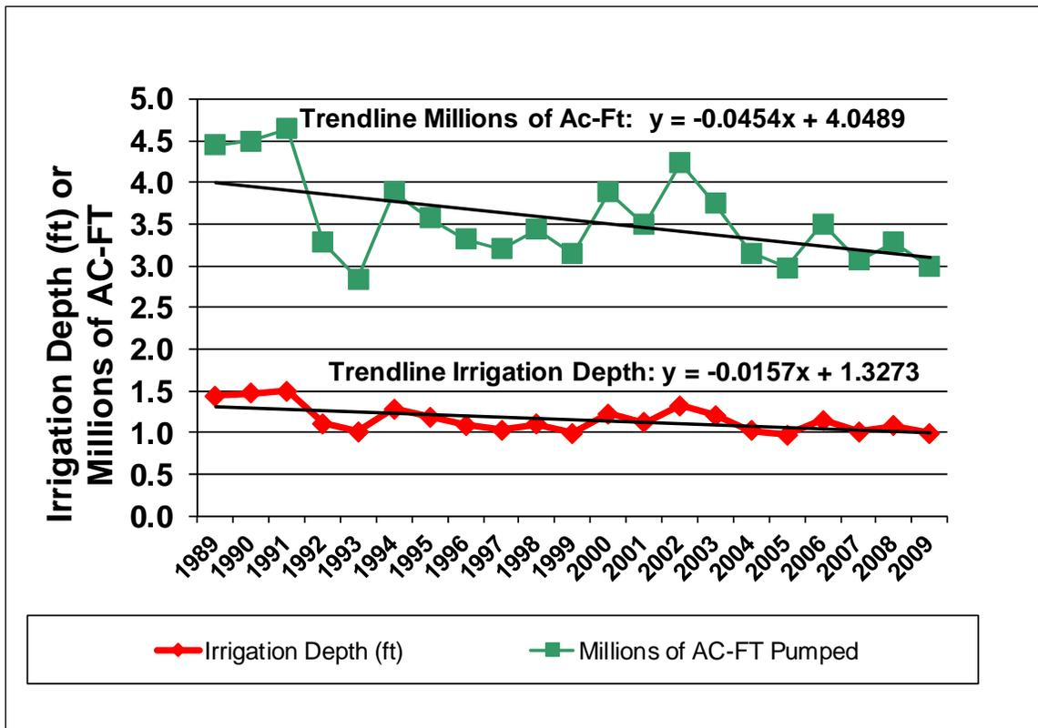
Figure 5. Total irrigation water diverted and average application depth by year for Kansas.
