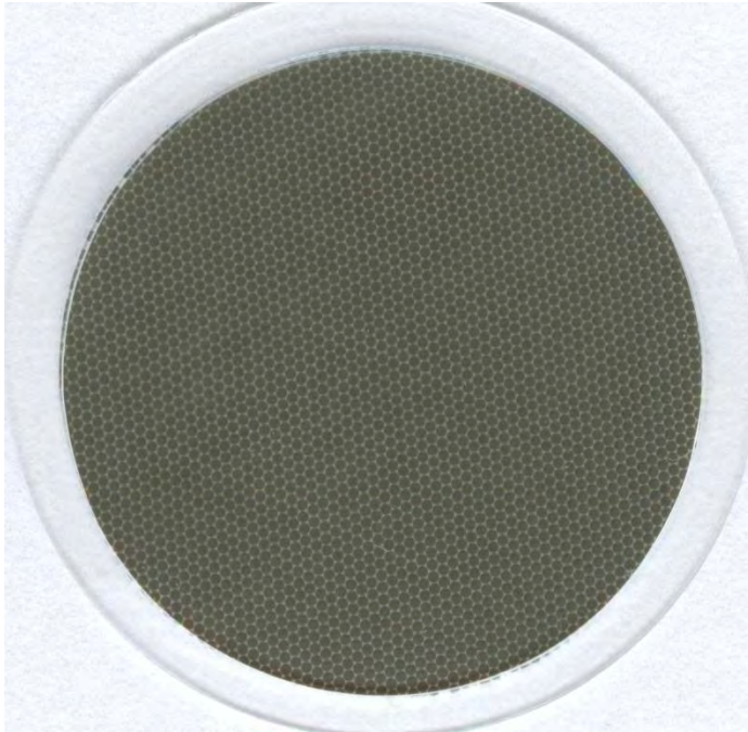
Figure 1.8. Filter sample collected using detached screen cassette.
