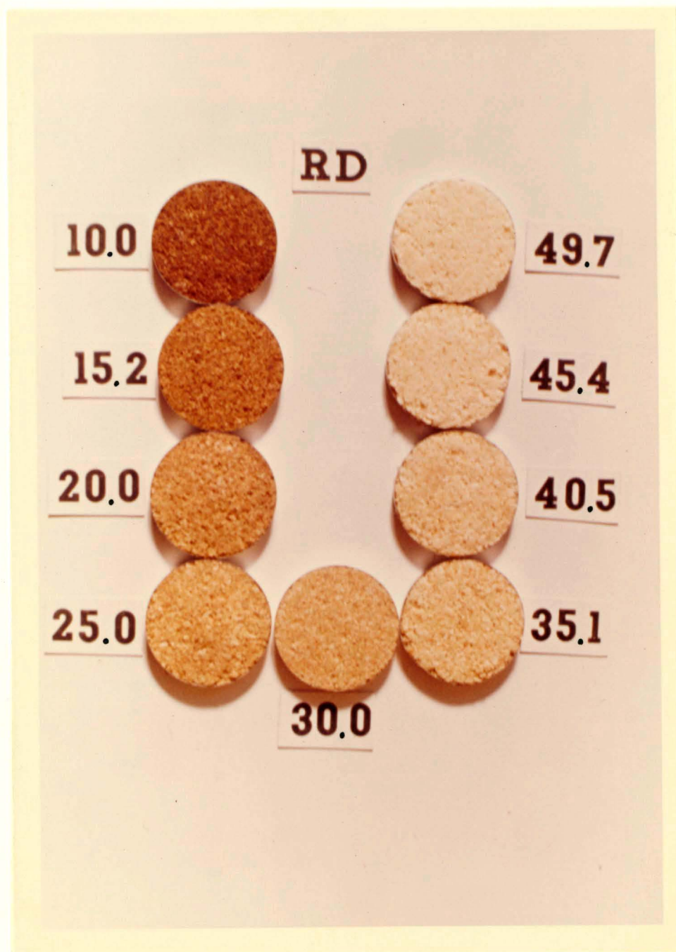
Figure 1.--The range of chip color that may be observed and their corresponding Rd value.
