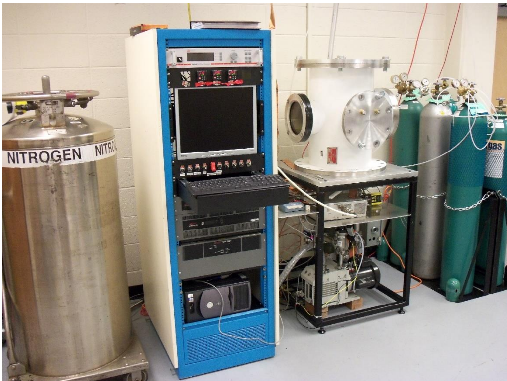
Figure 18 Picture of the RF sputtering system for MZO deposition.
