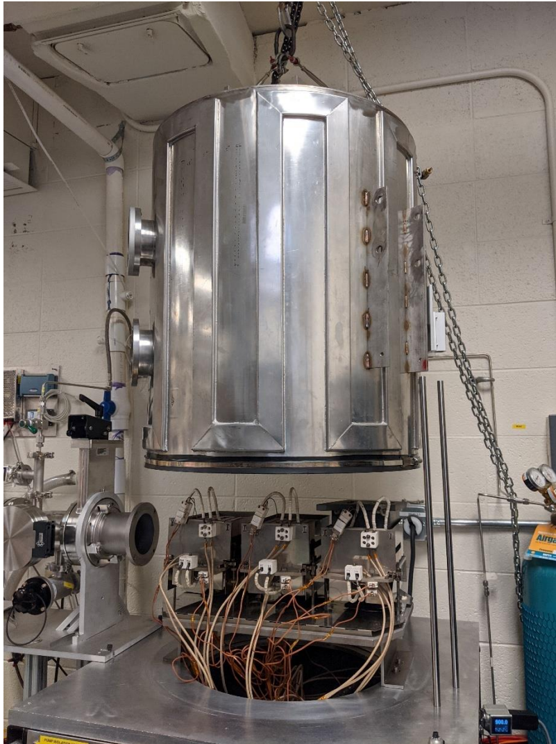
Figure 20 A picture of the CSS vacuum system for CuCl treatment.
